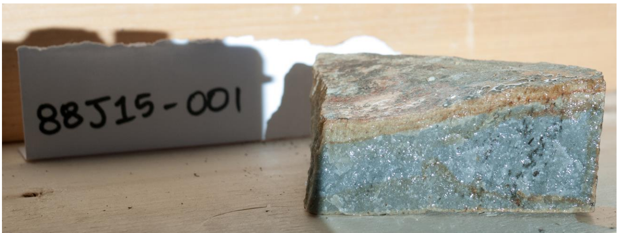
Picture 7: Sample 88J15-001 wet, note the disseminated, blebby sulphides.
