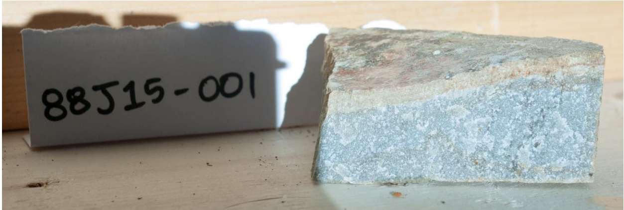
Picture 6: Sample 88J15-001 dry, note the disseminated, blebby sulphides.
