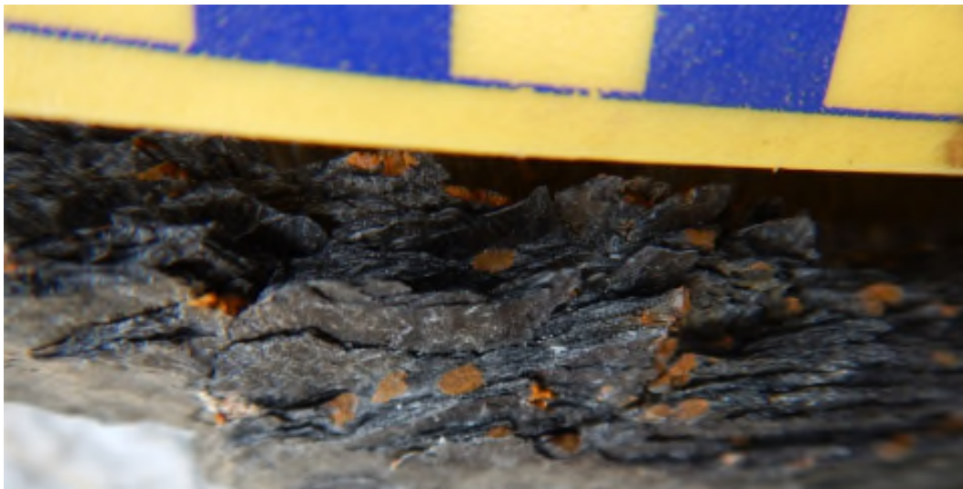
Figure 8. Photo showing fresh surface of graphitic, knotted phyllite broken across foliation. Note orange-brown Fe-carbonate porphyroblasts. Scale bar is in centimetres.
