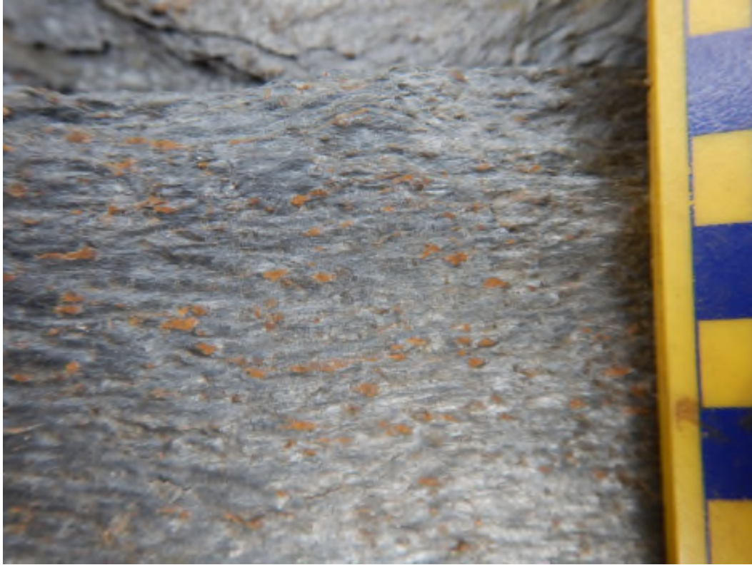
Figure 7. Photo of foliation plane in graphitic, knotted phyllite. Note abundance of knots (Fe-carbonate porphyroblasts) and lustrous sheen of surface. Scale bar is in centimetres.
