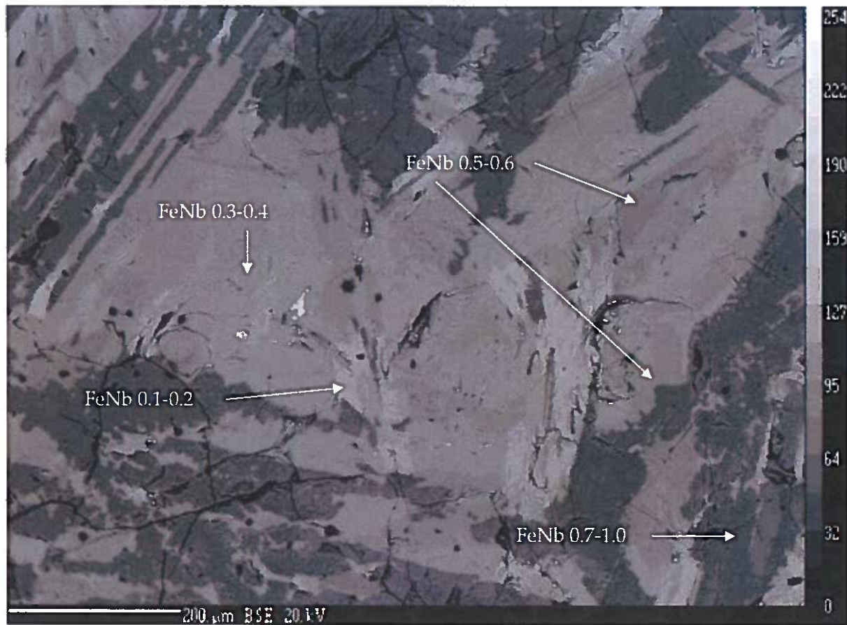
Figure 8: High resolution SEM images of the polished alloy surface.
