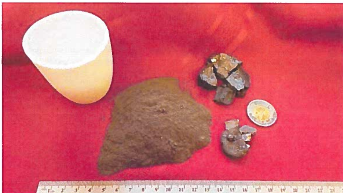
Figure 1: Scale of conversion tests: Crucible, charge, slag and alloy
