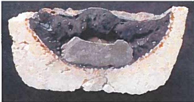
Figure 2: Image of Crucible, metal and slag for Run #3
