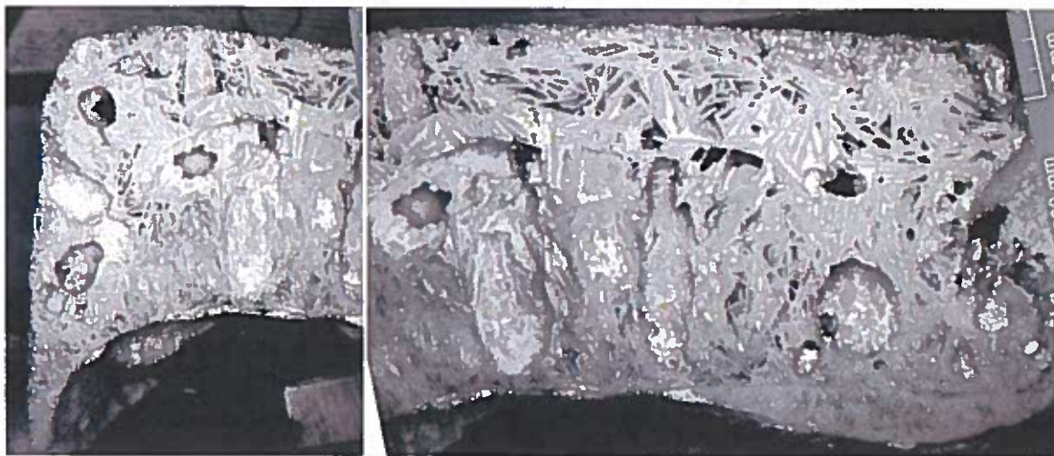
Figure 6: Comparison of the slag surface originally analysed and the new polished surface which the quantitative data is based on.
