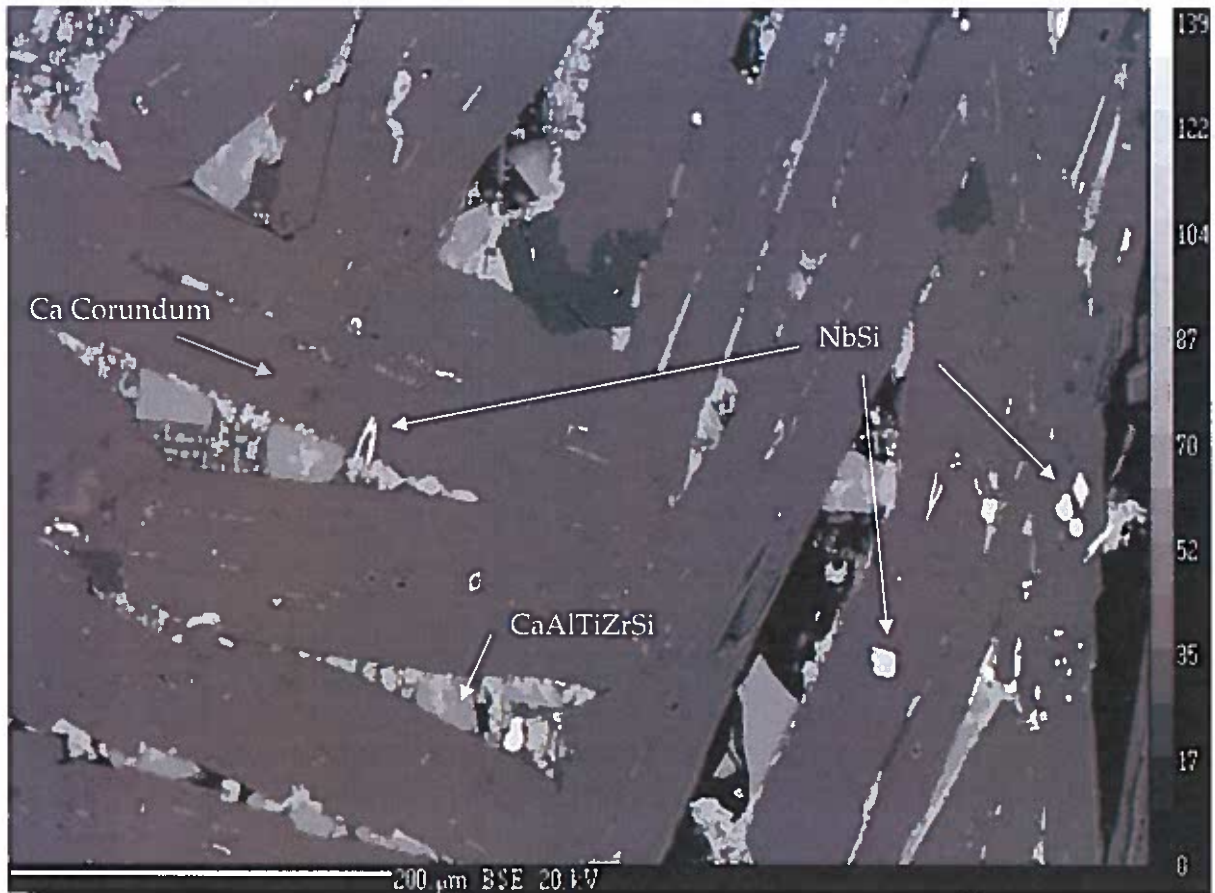
Figure 6: High resolution SEM image of the polished slag surface in increasing magnification showing the Ca corundum crystals with unreacted feed material trapped between them. The complexity of the trapped feed material is visible and shows why a consistent composition could not be obtained for each of the phases.
