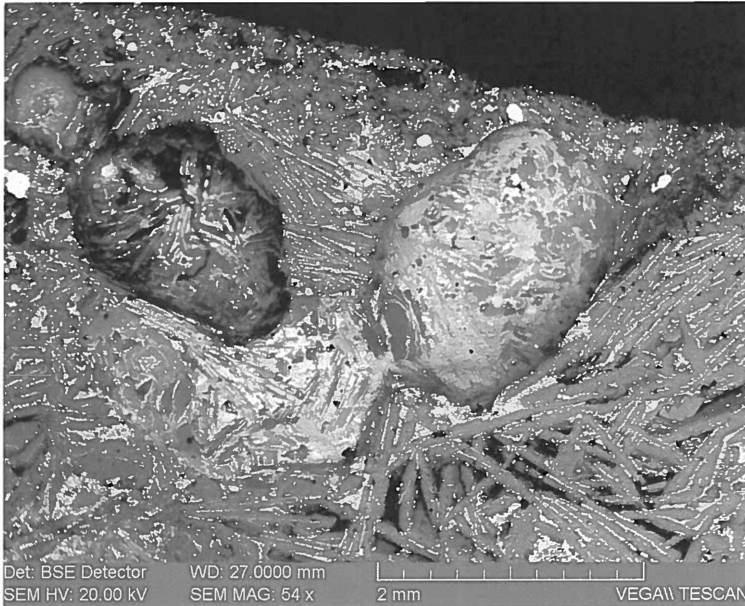
Figure 3: Closer view of side zone ( Again rotated relative to the original orientation). The small bright prills in the chill zone are visible.
