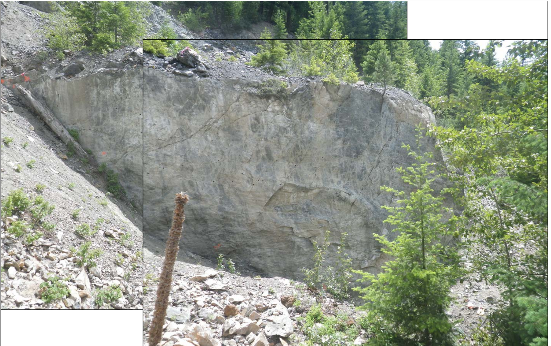
Figure 6: Photo of main workings showing the 7 m face of talc and nephrite (taken from the NW).
