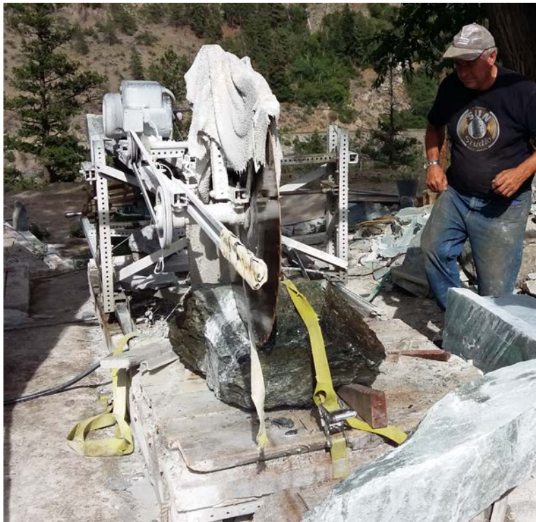
Figure 11: Large piece from the talc-nephrite layer being sawn.
