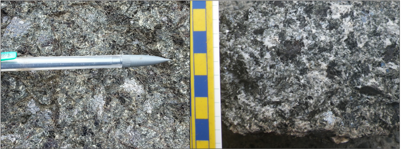
Figure 5: Dark grey to black, porphyritic, medium grained biotite-pyroxene gabbro.
