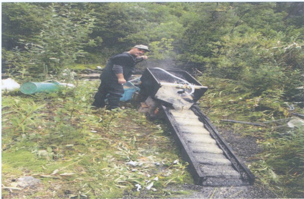
Photo#2 Mr. Vallee sluicing minus ½ gravels
