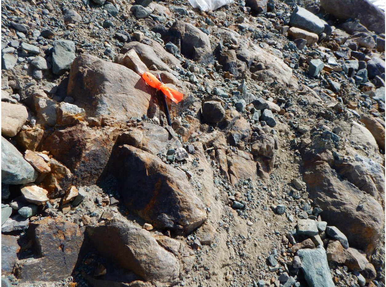
Figure 5: Chip sample location 2016SA903. Strongly oxidized and altered syenite with 10-15% fine grained disseminate pyrite. ICP assay returned significant values. 5.52ppm Au, 272ppm Cu, and 3.24Ag. Follow up location for 2015 sample.
