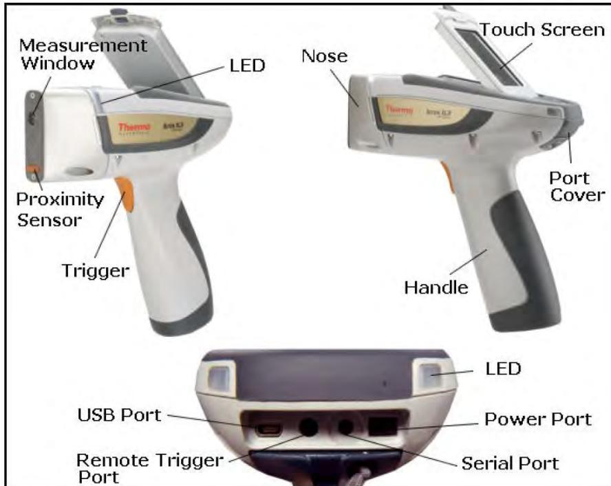
Overview of the Thermo Scientific Niton XL3t handheld XRF analyzer.
