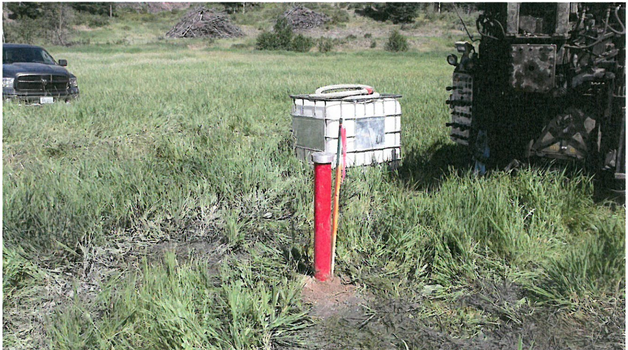
D.10: Standpipe installed at BH15-03N, Proposed Expansion Area.
