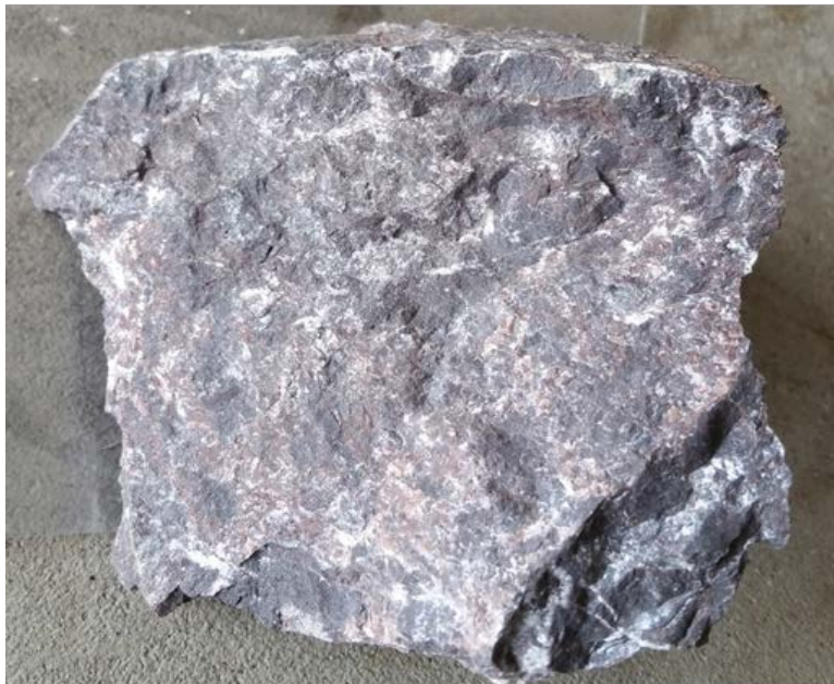
Photo 3 Brecciated and carbonate altered plagioclase-phyric basalt
