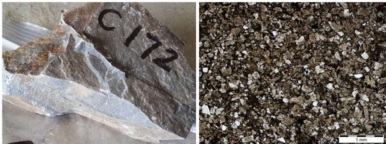
Photo 5 Fine-grained sandstone (specimen and micrograph)
