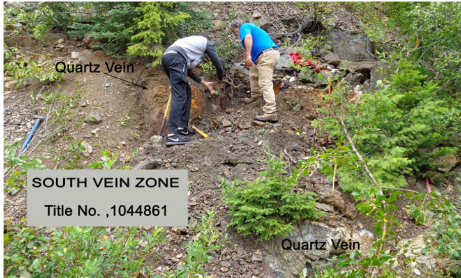
Two large Quartz vein systems are exposed along the 201 Forest Service Road (FSR) Mineralisation consists of Py, Ga, Sph, Cu-Py, and Tetrahedrite. Sample 663201 was taken from this trench. This is the most southern vein exposure. Quartz float indicates the zone continues south
