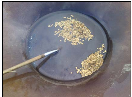
Figure 12D Panning Gold from Ironstone - 4
