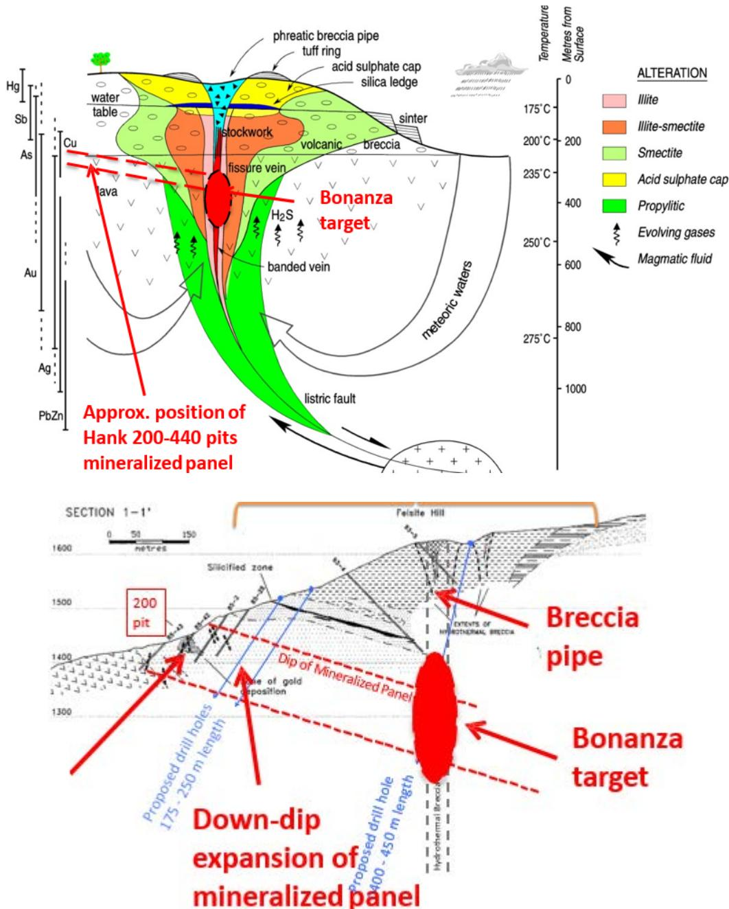
Figure 11.1 – Cross-sections of epithermal alteration model and Hank conceptual target
