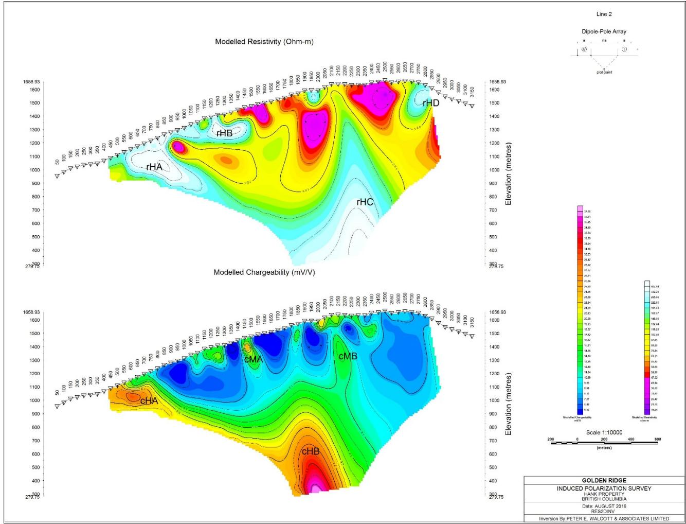
**Figure 10.10 – 2D Inverted Section Line 2**
