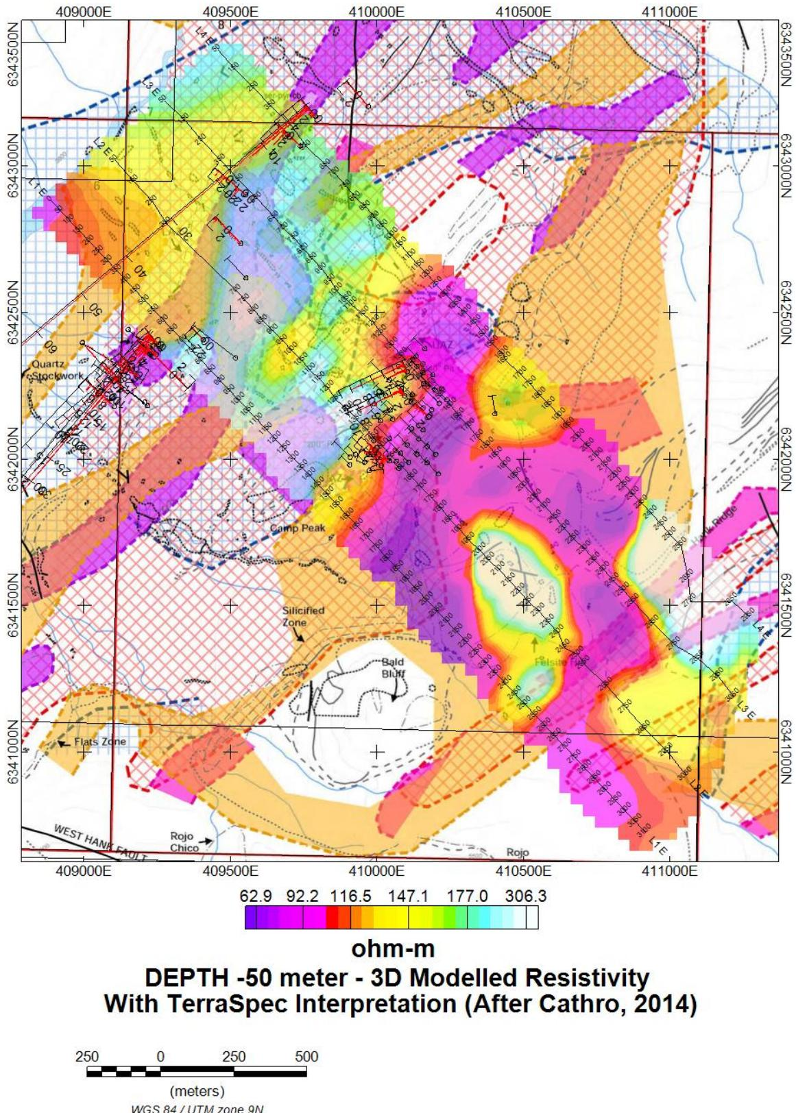
Figure 10.7 – 50 meter depth slice – 3D Modelled Resistivity
