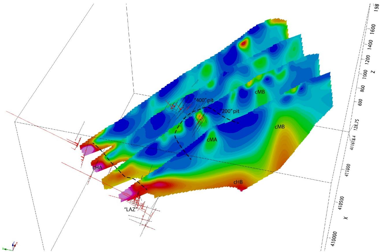
**Figure 10.6 - 3D View of 2D Modelled Chargeability**
