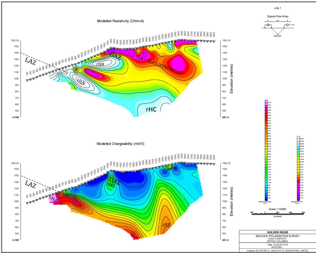
**Figure 10.11 – 2D Inverted Section Line 1**
