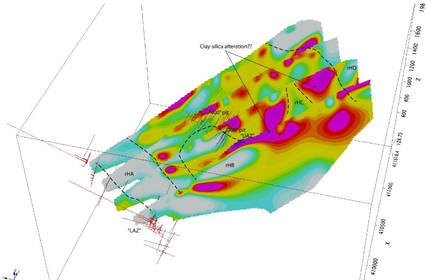
Figure 10.5 - 3D View of 2D Modelled Resistivity
