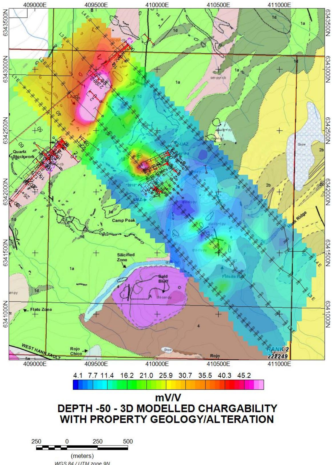
Figure 10.8 – 50 meter depth slice – 3D Modelled Chargeability
