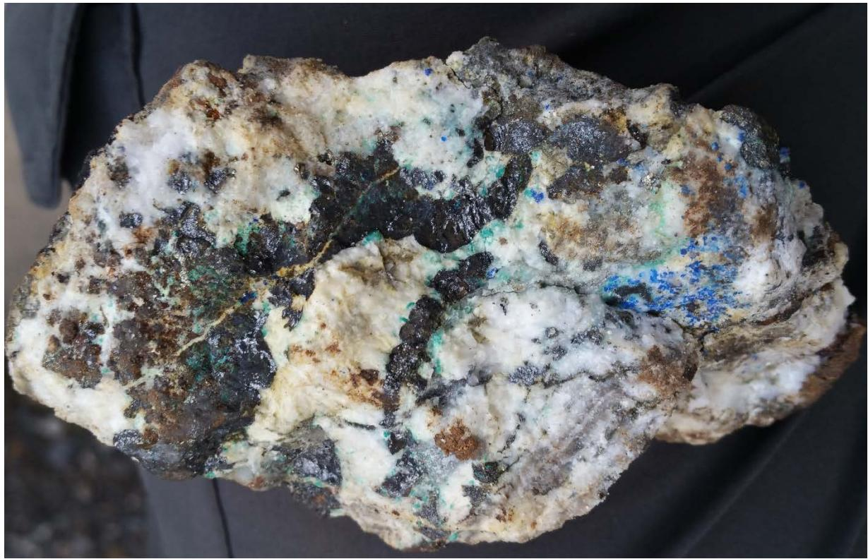
Photo 8 – Tetrahedrite-bearing quartz-calcite vein in 200 pit assaying 4790 g/t Ag, 25.8 g/t Au
