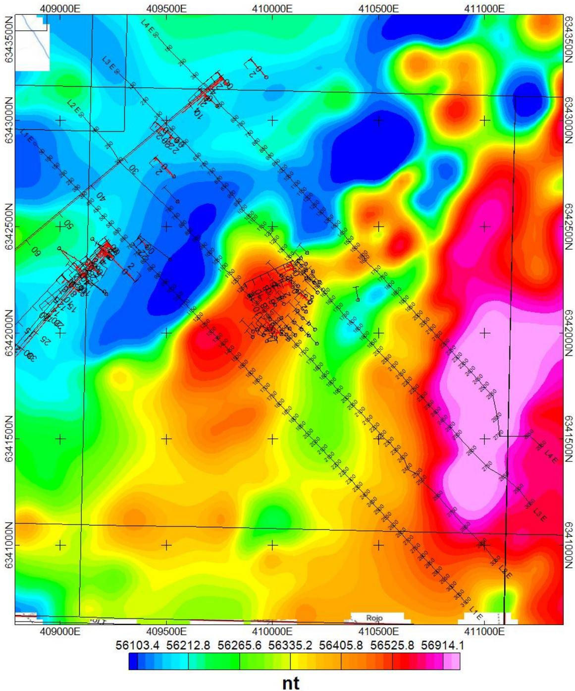
Figure 10.9 – Airborne Magnetics with Historic Drillholes showing Au values
