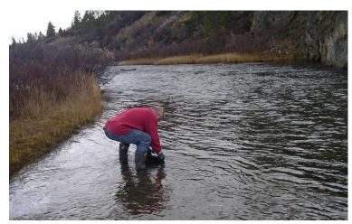
Panned material consisted of stream gravel, and was washed down to fines. Coarse materials were examined for any mineralization, quartz and rock types; fines were examined for placer gold and black sand.
