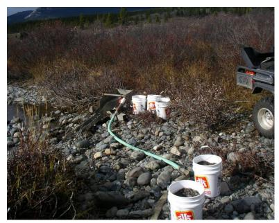
Each bulk sample was collected in five - 25 litre pails, (30 pails = 1 metre) from a hand dug hole approximately a metre deep. Sample material was then transported by ATV to a site on the river and run through a long tom and then processed by panning.
