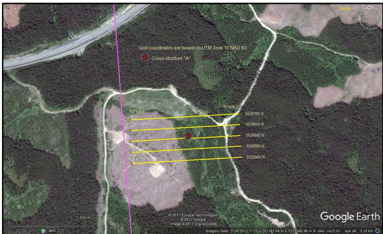
Figure 8. Magnetometer Survey Grid (Base map from Google Earth)
