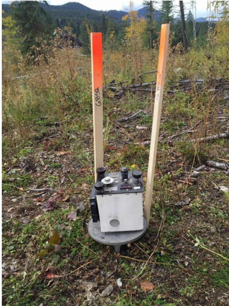
Figure 2. Lacoste and Romberg Gravity meter at base station
