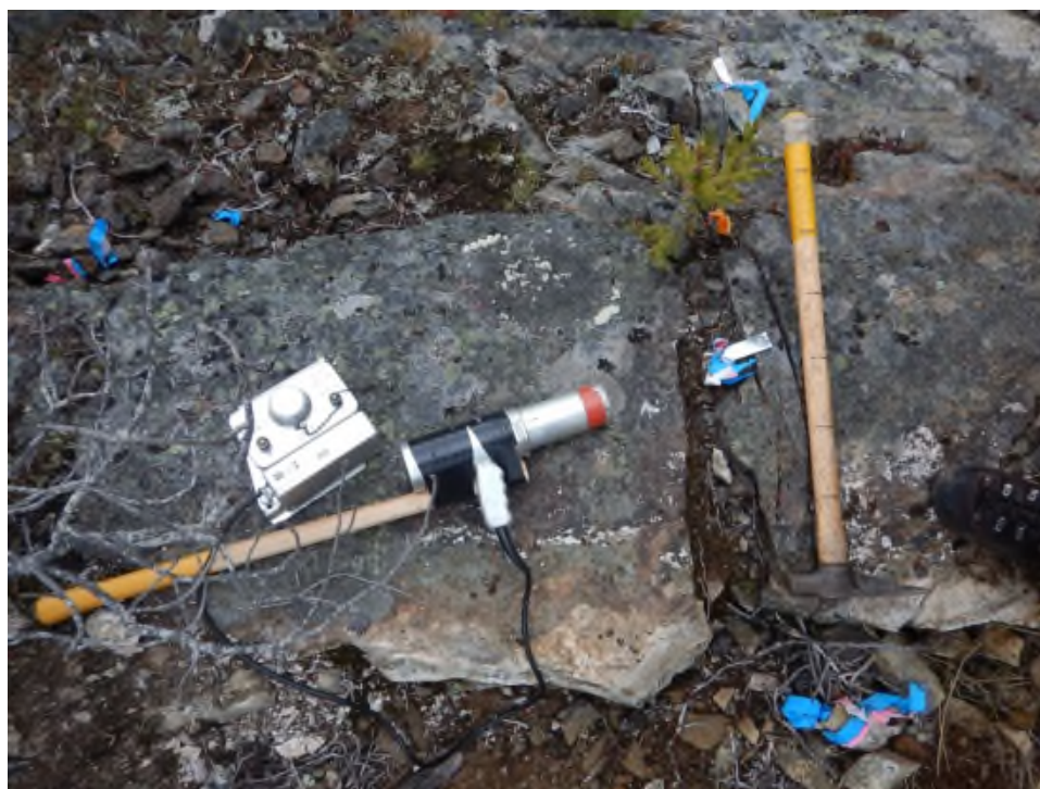
Figure 5. SRAT SPP2 scintillometer with wooden handle taped to detector.
