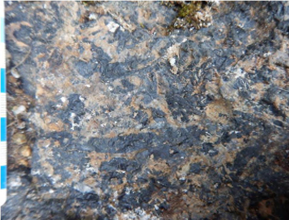
Figure 8. Close-up photo of vein containing abundant allanite (black crystals). Photo taken near UTM coordinates 438867E, 6156245N (close to trench 11-05). The blue intervals on the scale card on left side of photo are 1 cm long.
