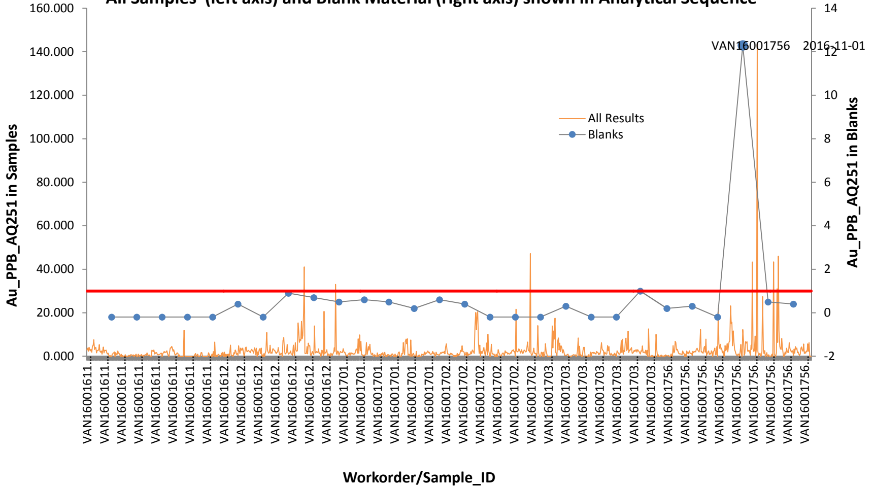
Chart 4: Chart showing gold values for blank samples analysed by AQ251 (15 g ICP)
