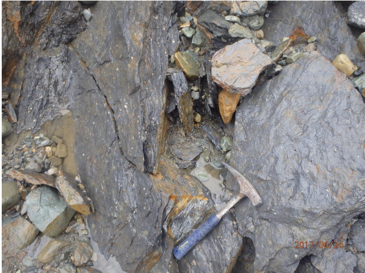
Figure 12 Pyritic phyllite striking 350 Az dipping west at 55°
