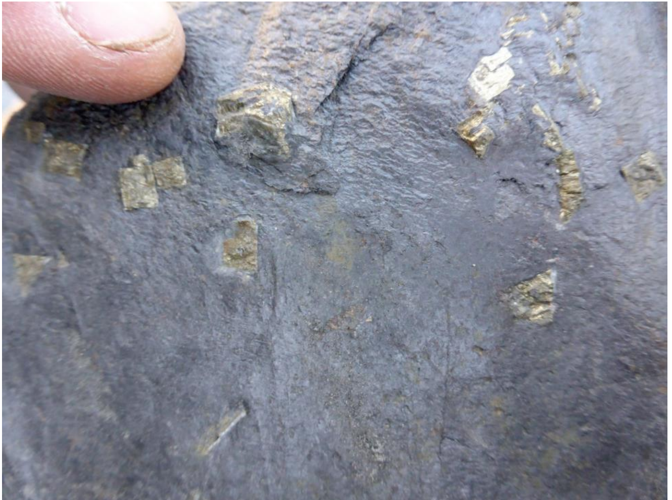
Figure 14 Black graphitic phyllite displays zones where coarse euhedral pyrite cubes and aggregates are common. Pyrite grains show fracturing, embayments and deformation to varying degrees.
