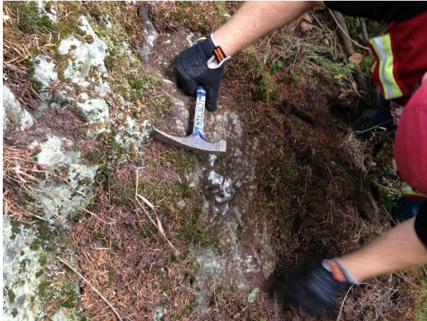
Small quartz vein, 5cm wide by 1.5 meters long, contains magnetite and minor pyrite.
