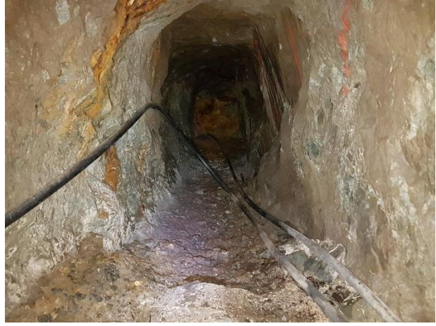
Start of the crosscut in the lower Jane adit, several samples containing chalcopyrite and sphalerite were obtained from the floor here.
