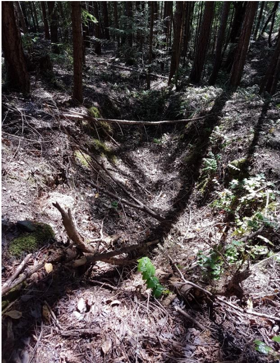
Trench near the old Jane workings. Five meters long, three meters wide and two meters deep. No mineralization was found in the trench.
