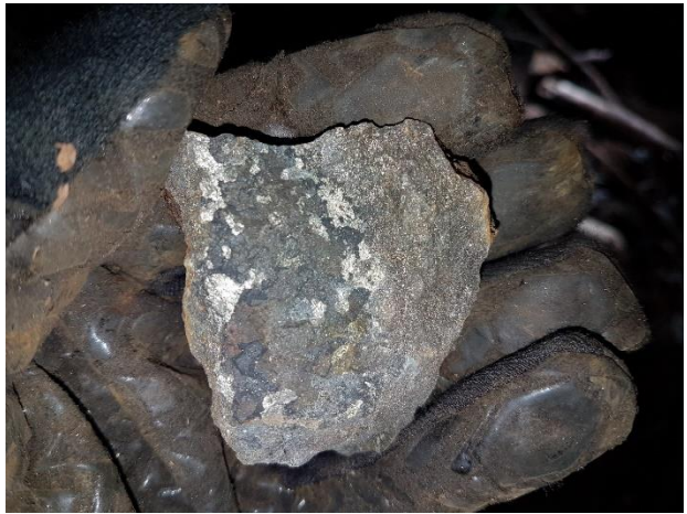
Samples removed from the lower mine dump pile. Contain sphalerite and chalcopyrite.
