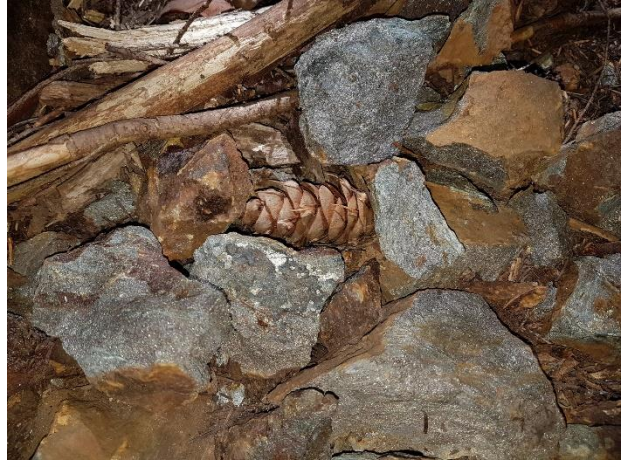
Samples broken from upper Jane adit mine dump. Sample contains sphalerite with chalcopyrite.
