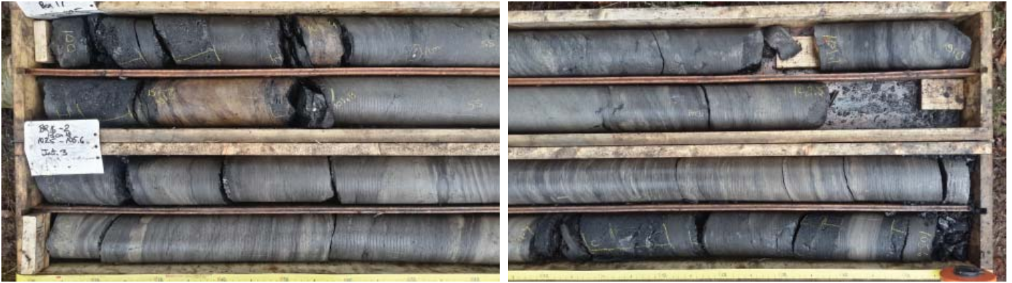
Figure 24: BR16-2; interval 3 boxes 17 and 18, 100 to 105.6 meters. Coal seam evident at start of core at 100 m.
