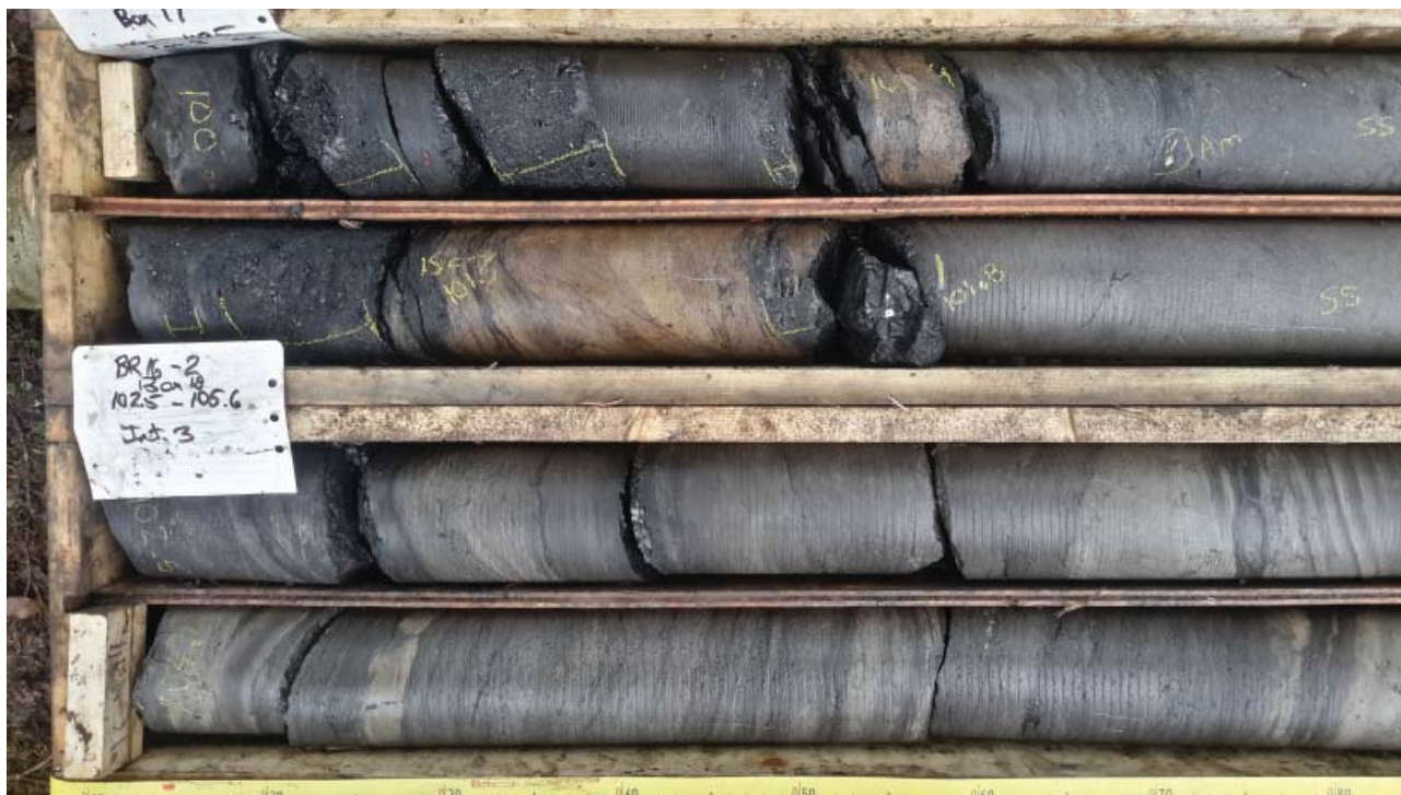
Figure 17: Start of third interval from 100 to 136 m showing coal and coaly shale. Reddish brown siltstones indicate oxidation. Flaser bedded siltstone-sandstones in bottom 2 rows.
