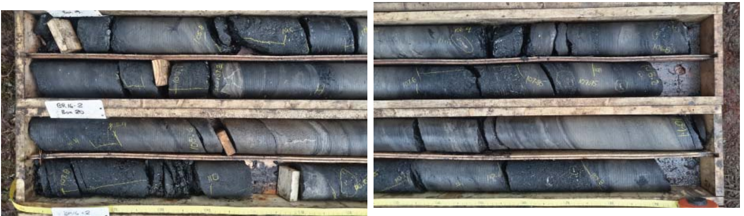
Figure 25: BR16-2, Int 3, Boxes 19 and 20, 105.6 m to 111.1 meters Several thin coal seams within sandstones and siltstones.
