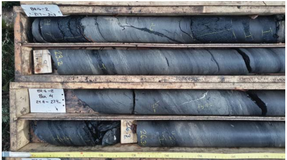
Figure 15: Thin coal seams near top of BR16-2. Flaser bedded siltstone and coaly shales intervene between coal seams.
