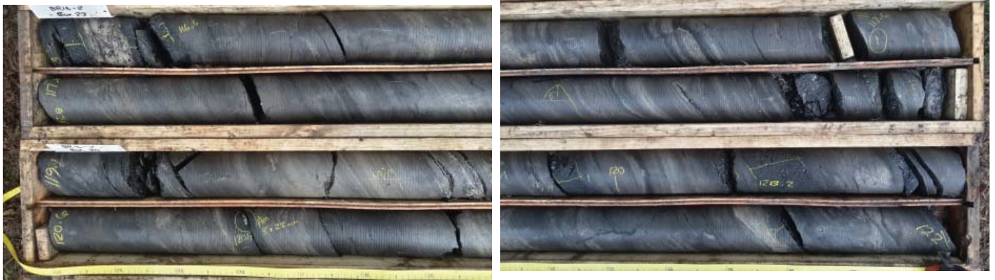
Figure 27: BR16-2, Int 3, Boxes 23 and 24, 116.3 to 122.0 meters. Siltstone and sandstone interbedded with coaly shale and minor massive coal.
