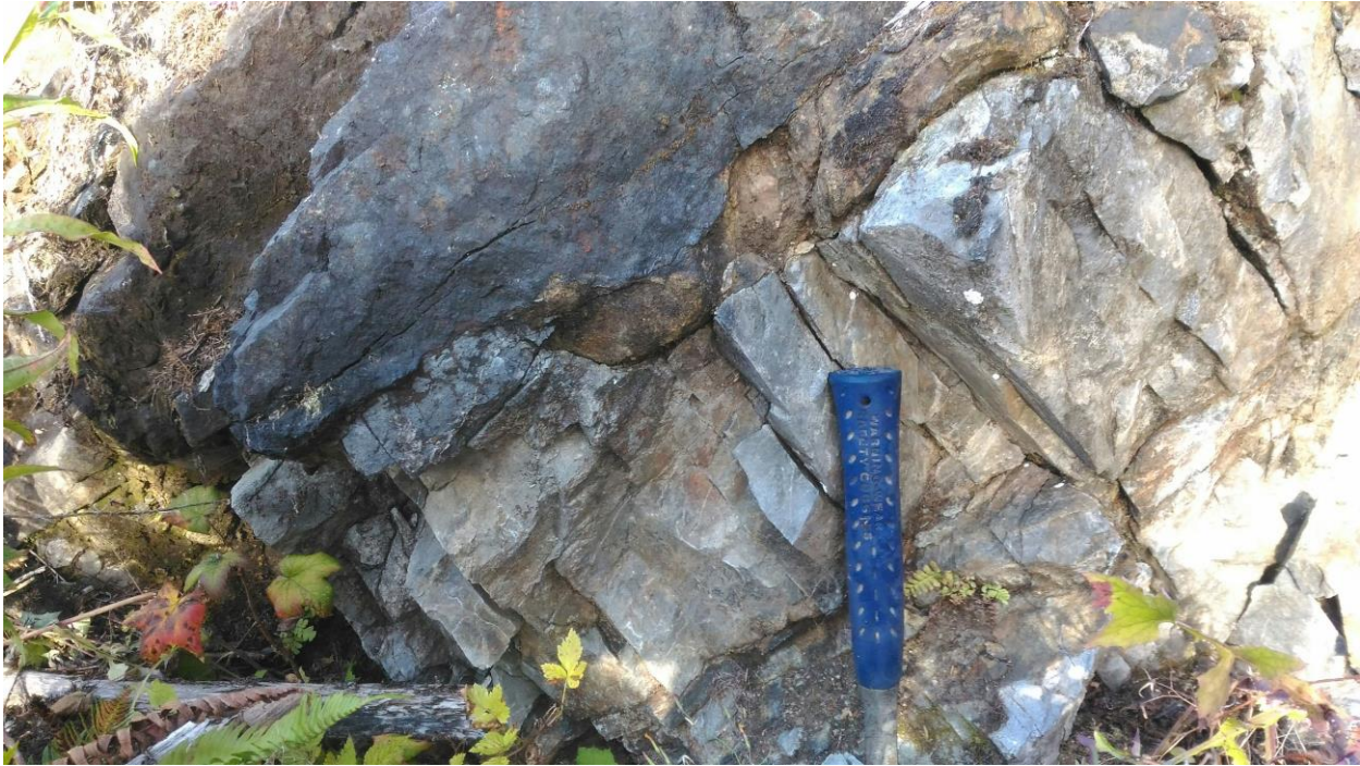
Figure 6: Magnetite skarn lens hosting disseminated and blebby pyrite and chalcopyrite at the West showing
