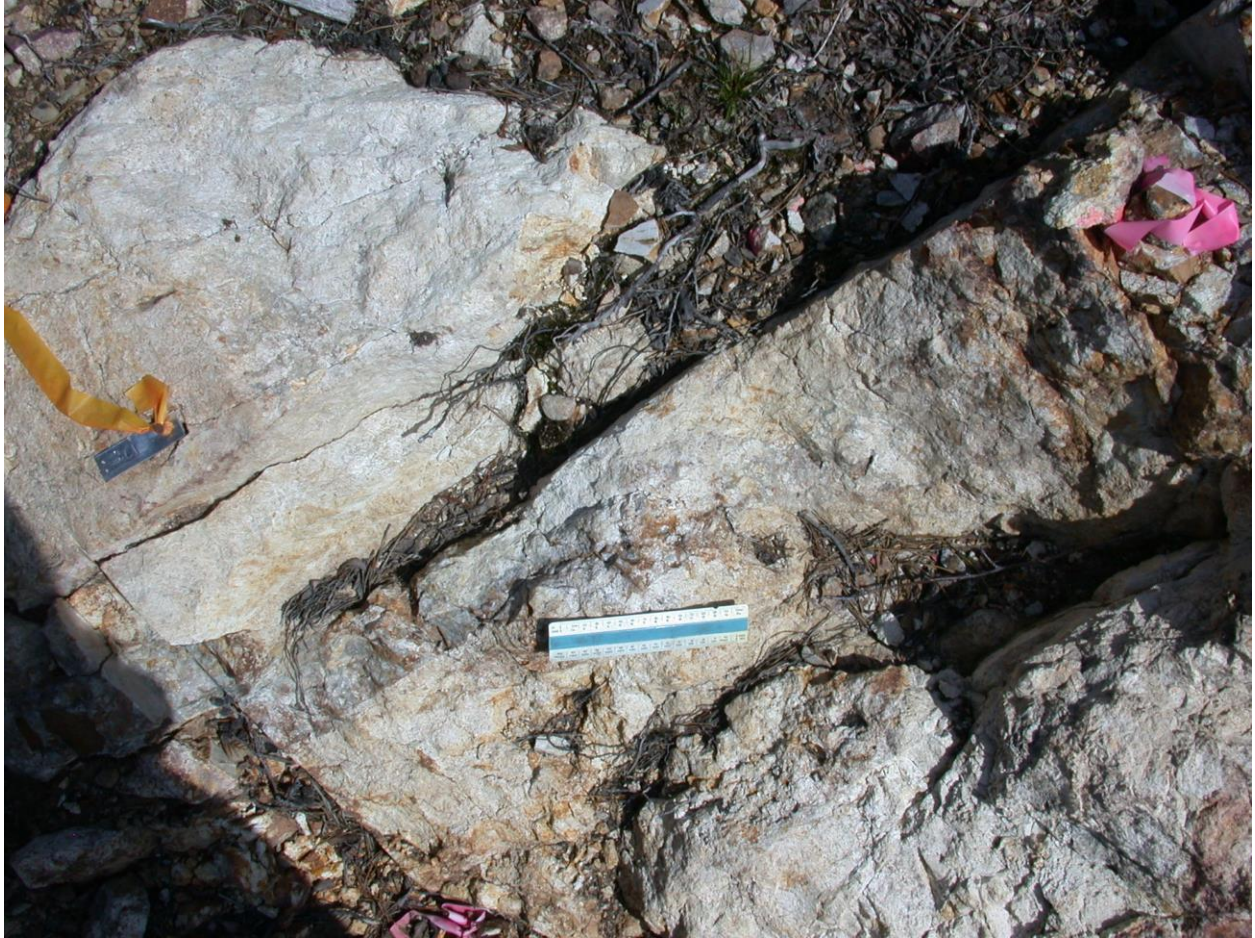
Fox C trench; NW end at historic sample FoxC1 (3 gpt Au). Later veins crosscut silica flood zone.
