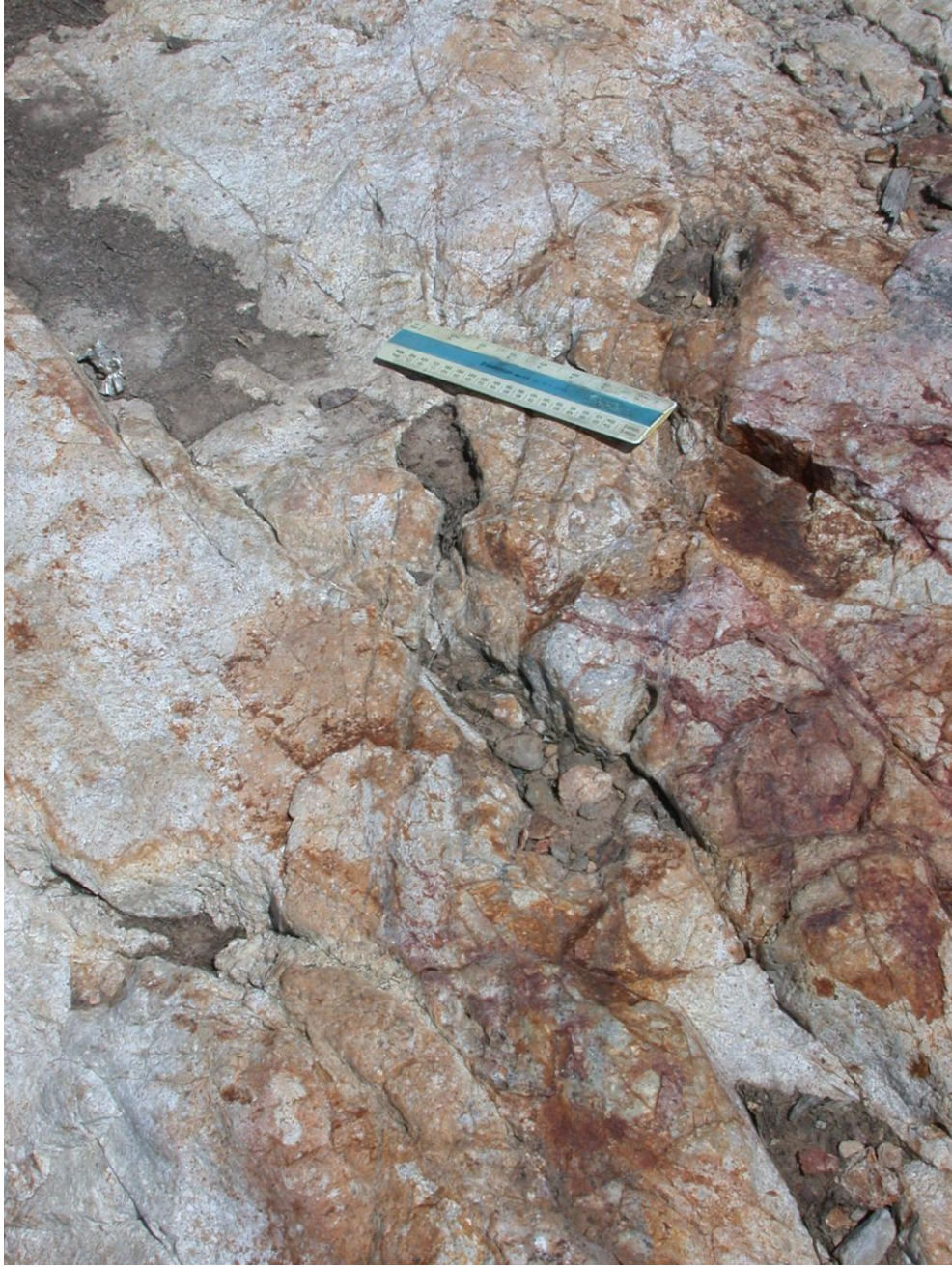
Fox E trench. Silica flooded zone exhibiting fragmental texture. Note later horse-tailing veinlets and limonitic fractures.
