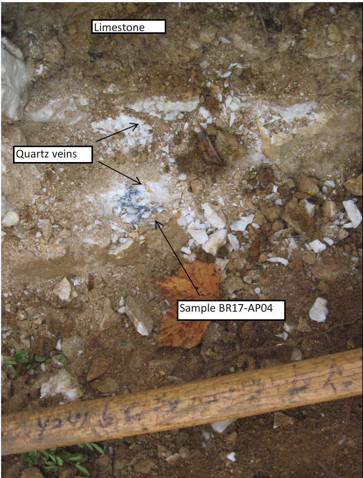
ILLUSTRATION #23: SILVERGAL Showing close up of Rock sample BR17-AP04 assayed Au 0.430 ppm; Ag 357 ppm; Bi 462 ppm; Pb 20 percent; S 3.04 percent; Sb 92.3 ppm; Zn 121 ppm (IMG_2445.jpg).
