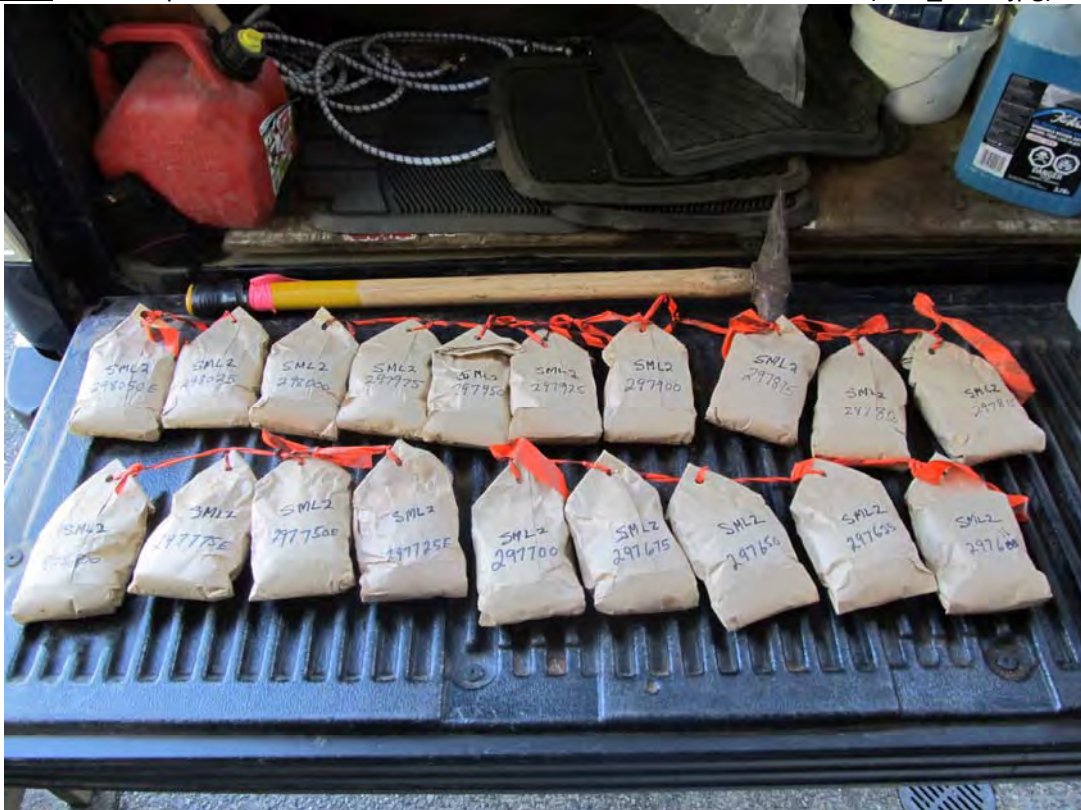
ILLUSTRATION #28: Soil Samples from the SILVER MINNOW GRID SML2 –Line1 in 2017. (IMG_2001.jpg).
