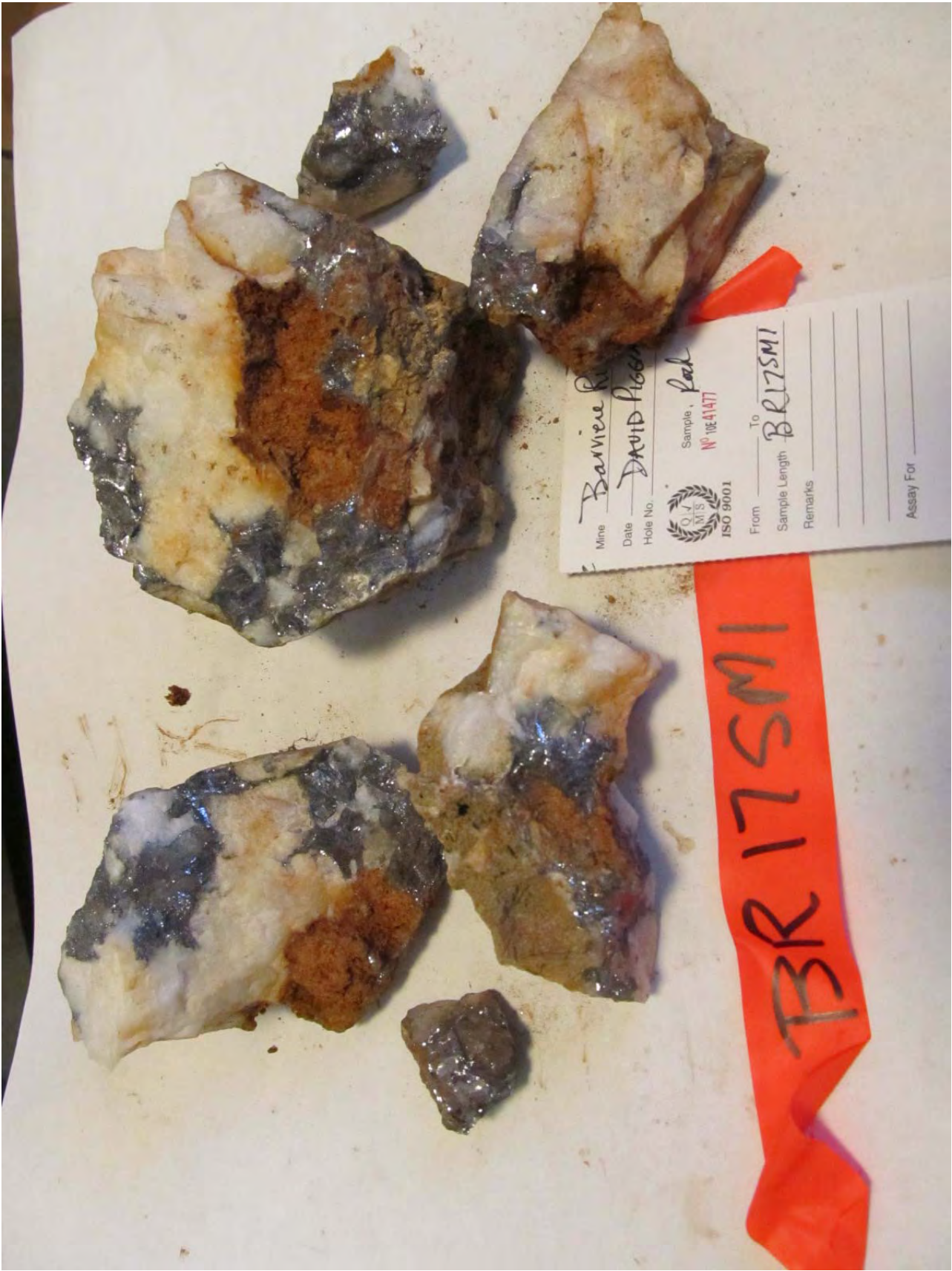
ILLUSTRATION #24: Rock sample 10E41477_BR17SM1 from the SILVER MINNOW MINFILE assayed Au 0.11 ppm; Ag 308 ppm; Pb 20 percent; S 3.04 percent; Sb 277 ppm; Zn 1.23 percent (IMG_2032).
