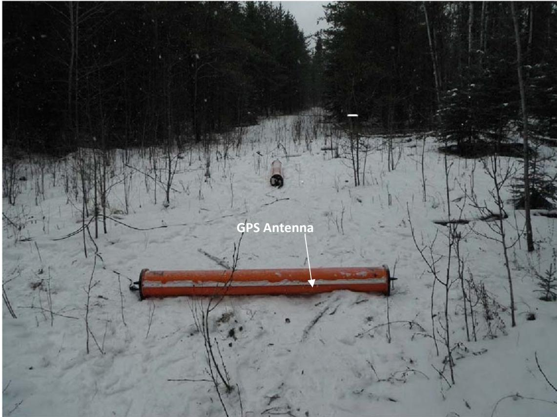
Figure 7: ZTEM base station receiver sensor.
