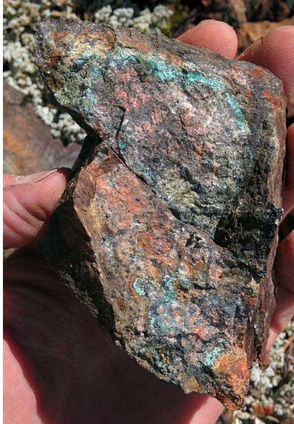
Figure 6: Magnetite-chalcopyrite with pink K-feldspar
