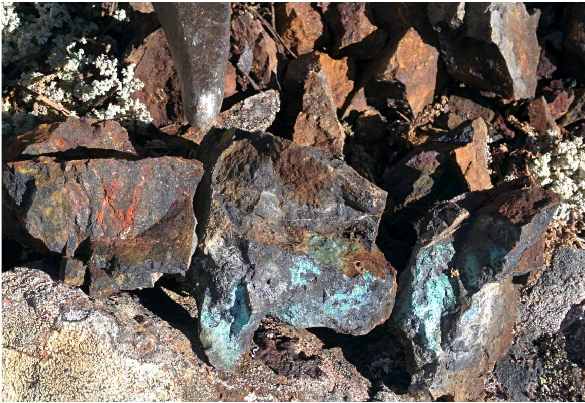
Figure 5: Malachite stained poddy semi-massive magnetite and sulfides, Vector showing.
