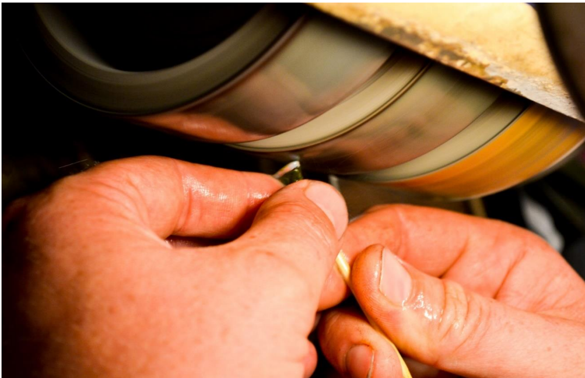
Opal cutting and processing is conducted using diamond saws, diamond grinding and polishing wheels.
