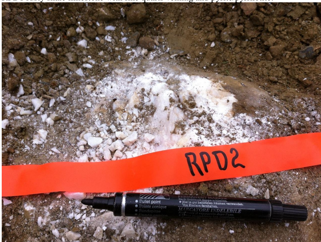
RPD2 Quartz float some very fine grains of pyrite- barren for the most part.
