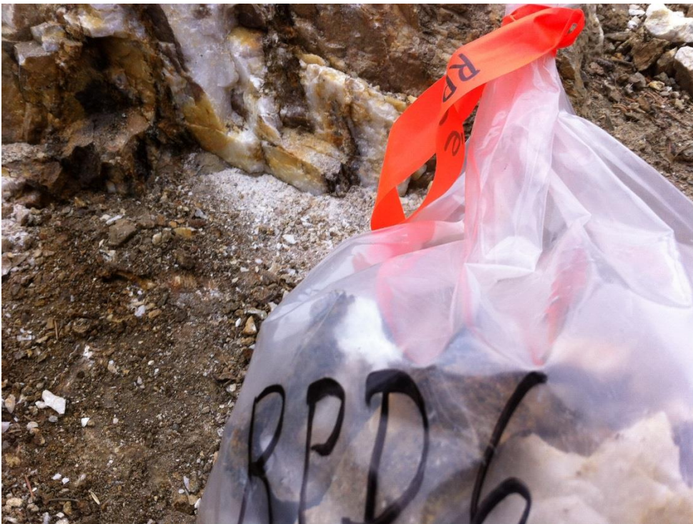
RPD6- quartz vein with rusty thin 1-2 mm wide seams (veins). Small pieces of pyrrhotite found in some of the seams.
