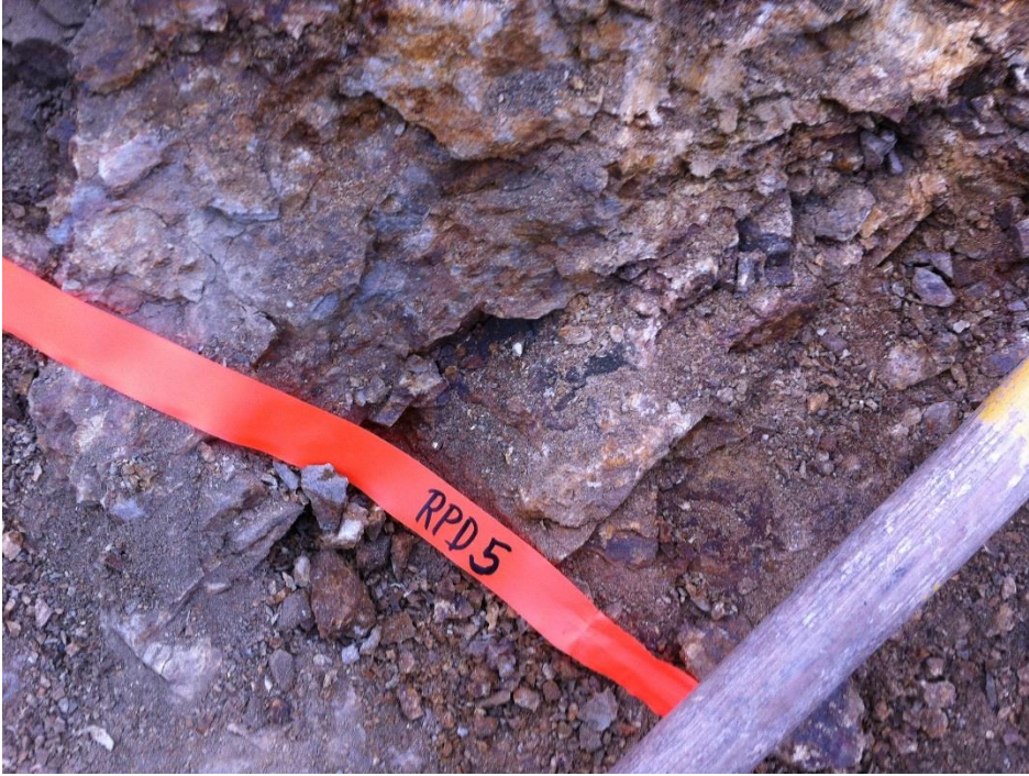
RPD5- Out crop of shale limestone tan colored rotten- interspersed by a pyrite/pyrrhotite veins.
