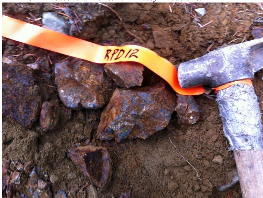
RPD12- float- very heavy mafic limestone mineralized with iron pyrite and small specks of chalcopyrite.
