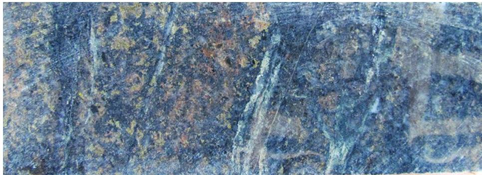
**Figure 10-6: JY17003 @ 442.2 m, hematized, epidote-dark chlorite-magnetite altered intermediate dyke porphyry (IDP2) with disseminated honey coloured sphalerite and irregular quartz-magnetite veinlets with honey coloured sphalerite. The 3 m interval (442-445 m) hosting this sample yielded 7,080 ppm Zn**
