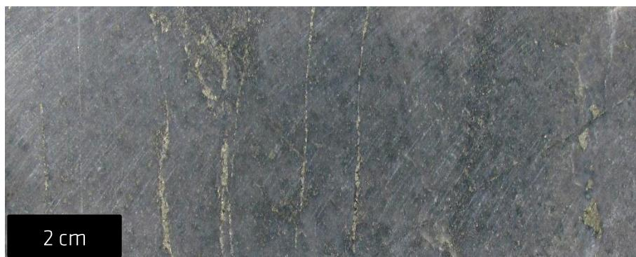
*Figure 10-4: JY17002 @ 444.20 m, strong to intense quartz-pyrite altered fine intermediate volcanics (IVC1) hosting a set of pyrite stringers. The 3 m interval (444.2-447.2 m) yielded 0.010% Cu, 152 ppb Au, 5.5 ppm Ag, 45.7 ppm Mo and 600 ppm Zn*
