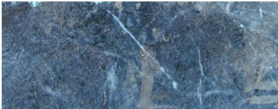
**Figure 10-7: 17003 @ 469.2 m, moderate dark chlorite-epidote-magnetite altered intermediate porphyry dyke (IDP2 hosting stringers and blebs of sphalerite and pyrite. The 3 m interval (467.63-470 m) hosting this sample yielded 160 ppb Au and 1.7% Zn.**
