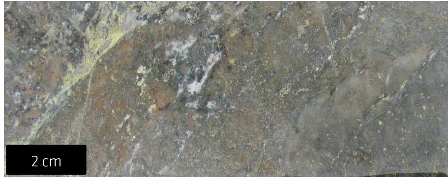
**Figure 10-5: JY17002 @ 462.23 m, strong quartz-pyrite and epidote-chlorite-pyrite altered fine intermediate volcanics (IVC1) hosting a set of pyrite stringers. The 3 m interval (462.2-465.2 m) yielded 0.010% Cu, 95 ppb Au, 1.2 ppm Ag, 7 ppm Mo and 160 ppm Zn.**
