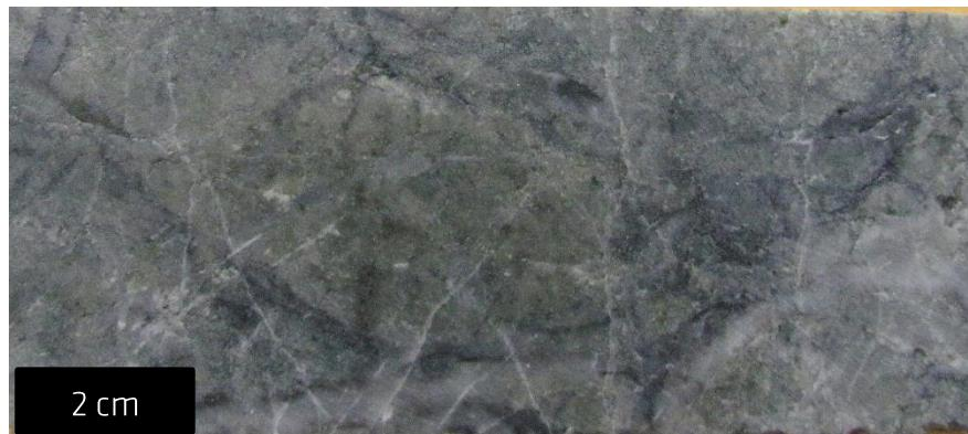
**Figure 10-2:** JY17001 @ 248.7 m, strong to intense quartz-pyrite altered intermediate dyke porphyry (IDP1) with dark quartz-magnetite veinlets. The 3 m long interval (248-251 m) hosting this sample returned 0.088% Cu, 63 ppb Au, 1.6 ppm Ag, 150 ppm Mo and 140 ppm Zn
