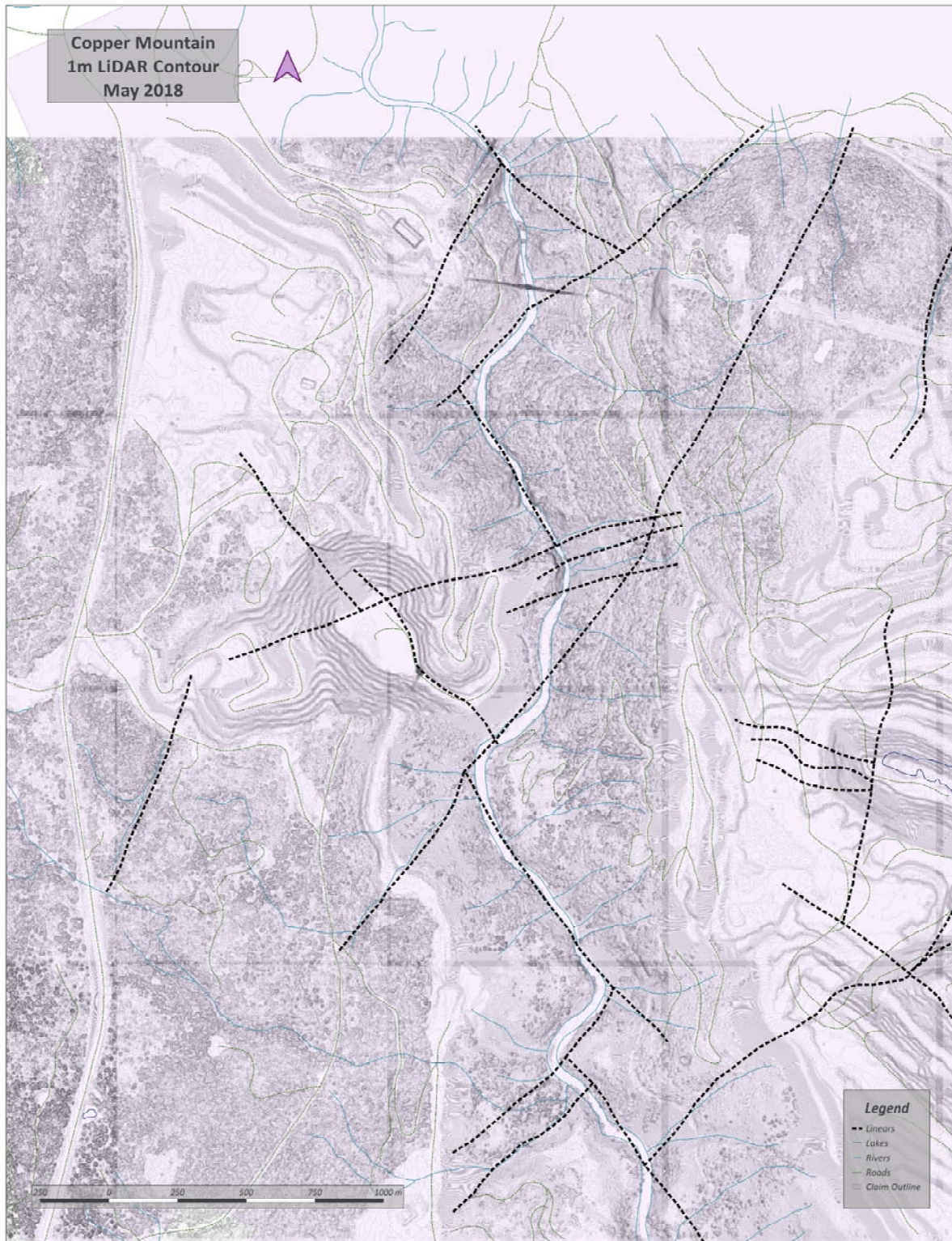
Figure 2.4: Image of 1m contours from Lidar Survey, interpreted fault structures denoted by dashed lines. Full size image below
