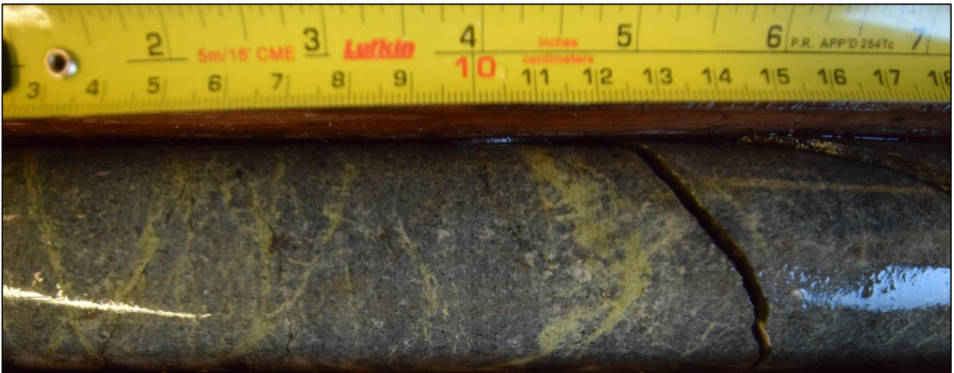
Plate B: Granodiorite with pervasive chlorite alteration and quartz-carbonate-epidote veins with epidote alteration envelopes. DDH Grand 10-05, 94.04 m.
