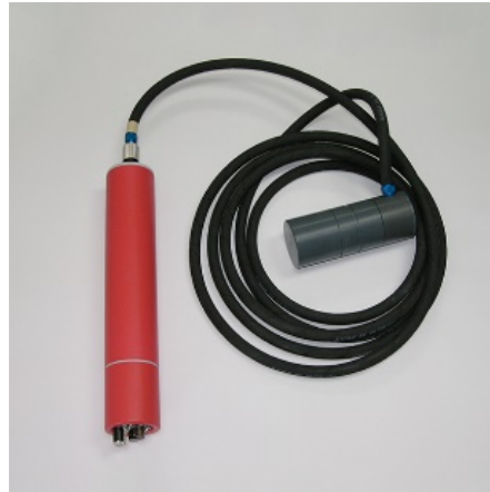
Figure 7 - The Scintrex CS-3 sensor with cable and driver electronics.
