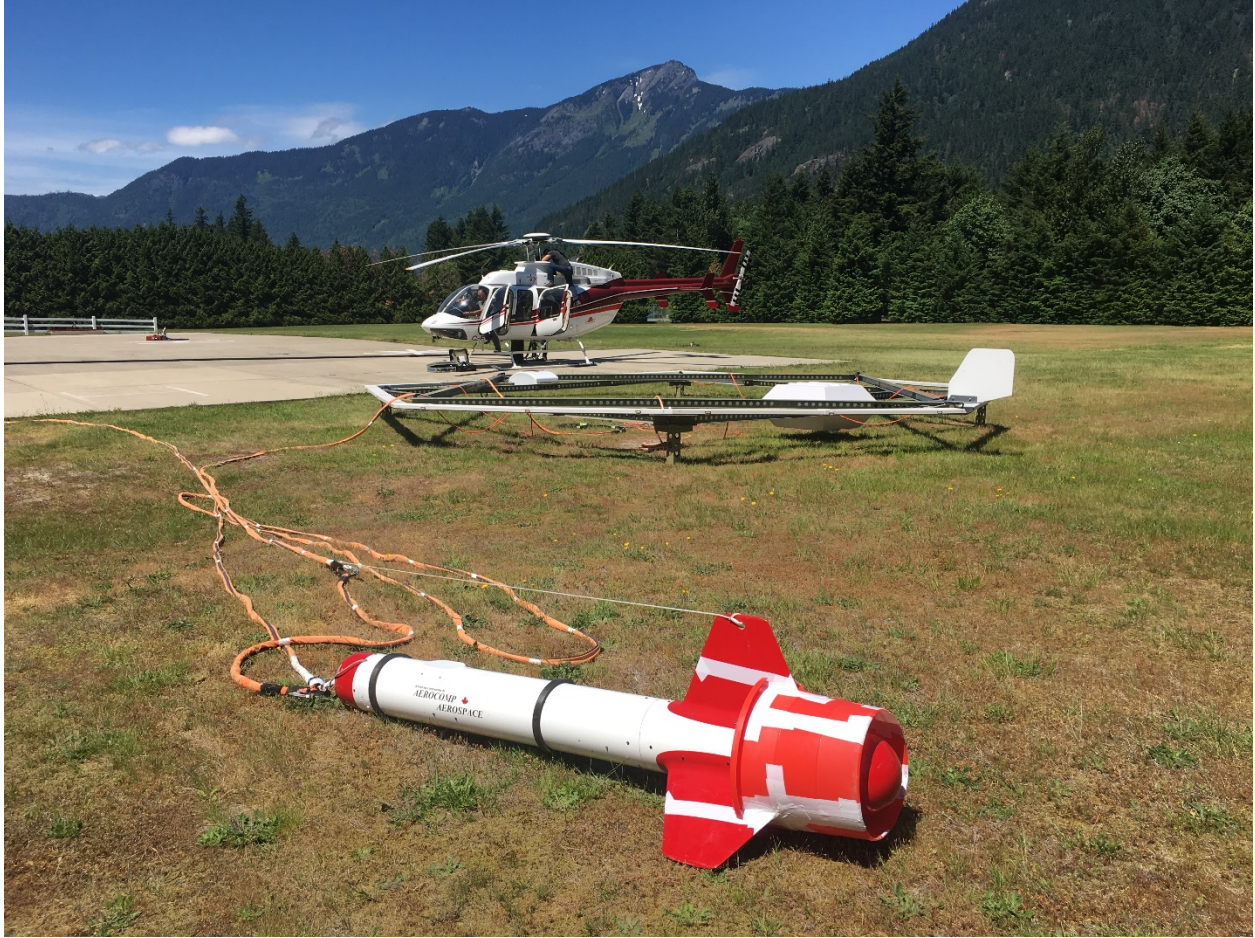
Figure 5 - The AirTEM system (background) with magnetometer bird (foreground).
