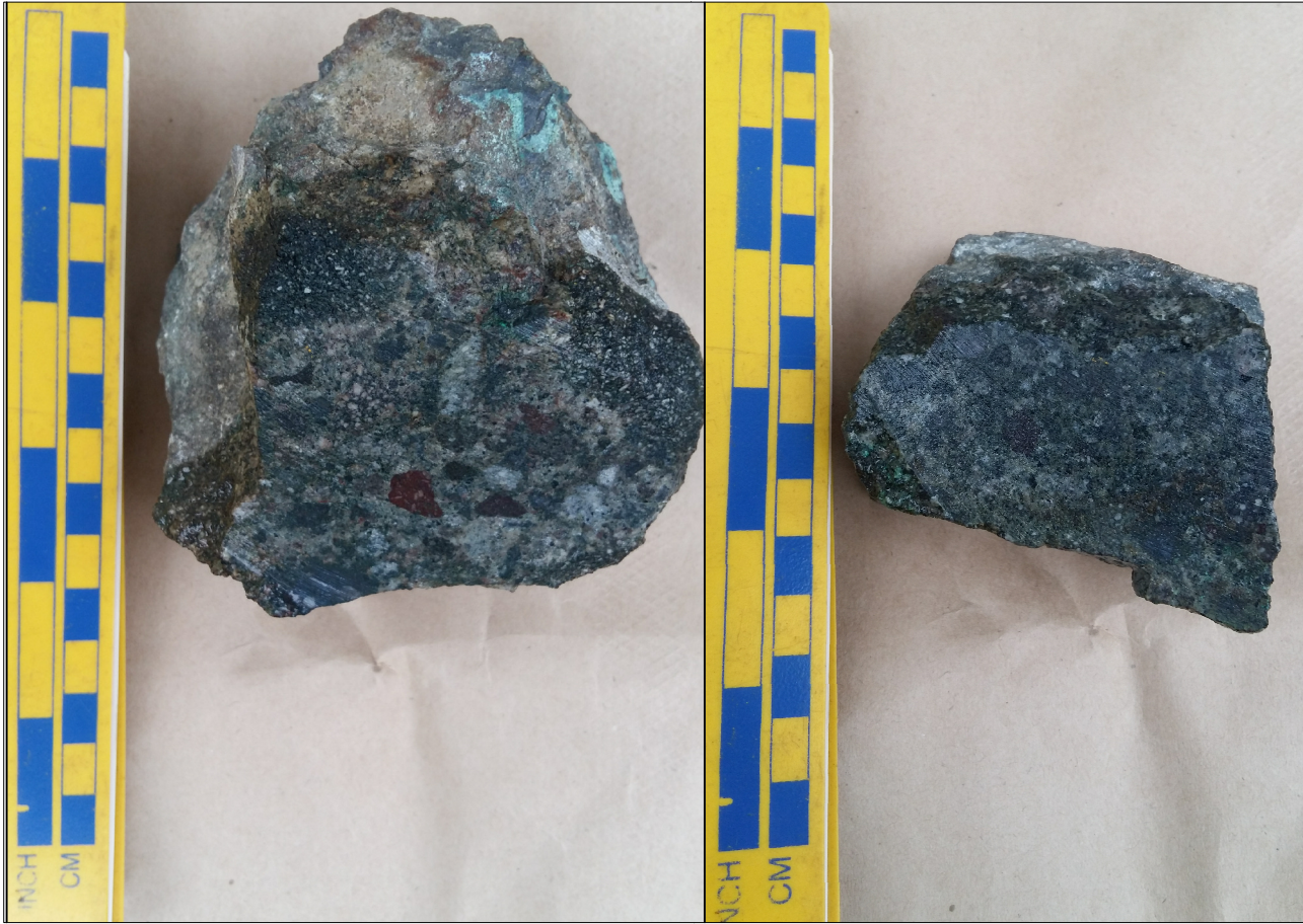
Figure 5: Volcanic conglomerate with chalcocite clots and malachite staining from the Tom Cat Showing.
