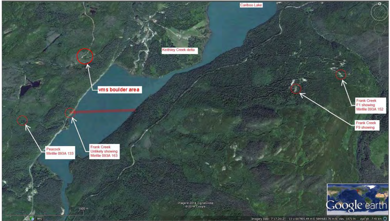
Figure No. 9. Satellite photo of approximately the same area as in Figure No. 8. An east-west topographic lineament, located on the south side of the Frank Creek F1 and F9 showings, extends westward toward the Unlikely showing. The lineament is plainly evident over the land area across the centre of the photo and is partly indicated by a red line drawn only over the lake. A portion of the Unlikely showing outcrop has intense shearing (see Figure No. 10) indicating an east-west fault with a vertical dip which may be related to the above lineament. The proposed E-W fault may pre-date the NE-SW fault (or joint) occupying the Cariboo Lake valley as the latter fault line shows no significant displacement in an E-W direction. Likewise, the proposed E-W fault also appears not to be displaced as it's line crosses the Cariboo Lake valley undisturbed. This, and the regional geology, suggest no great strike-slip movement occurred along the NE-SW line. It is possible the Unlikely mineral occurrence to the west are equivalent to the F1 and F9 occurrences at Frank Creek, displaced by an E-W fault.
