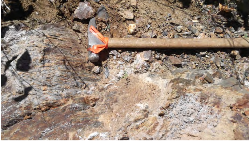
Figure No. 10 Vertically-dipping east-west intense shear at the Unlikely showing.
