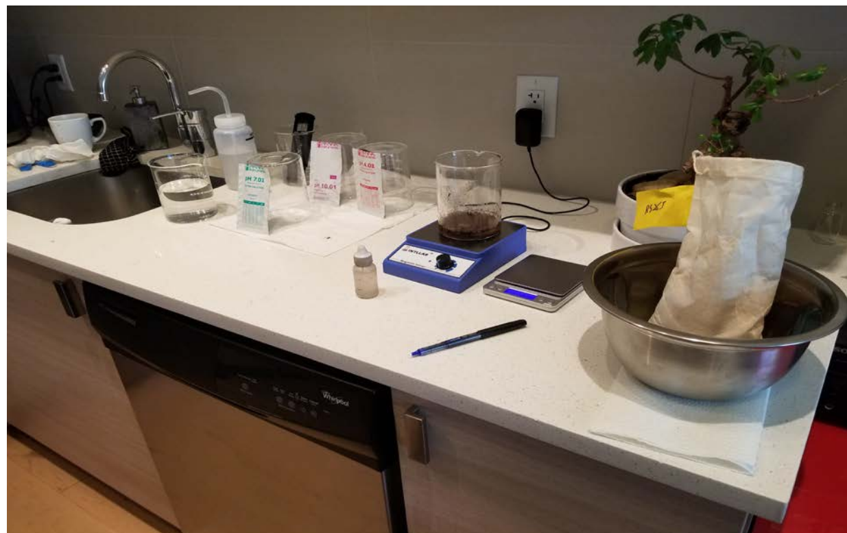
Figure 8: Analytical Setup for pH, pHa and Conductivity
