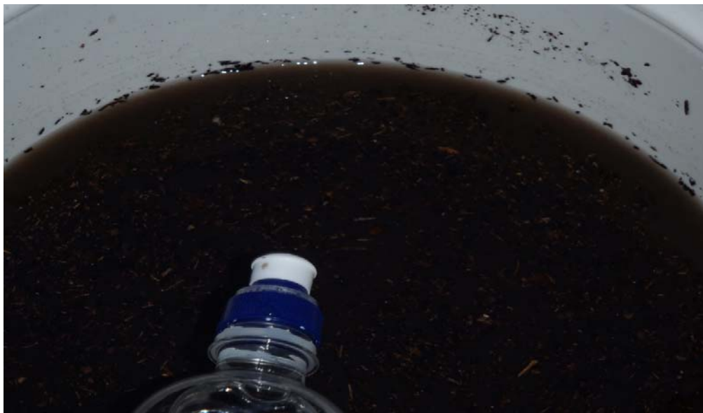
Figure 3 showing early sign of flocculation at edges of plastic container.
