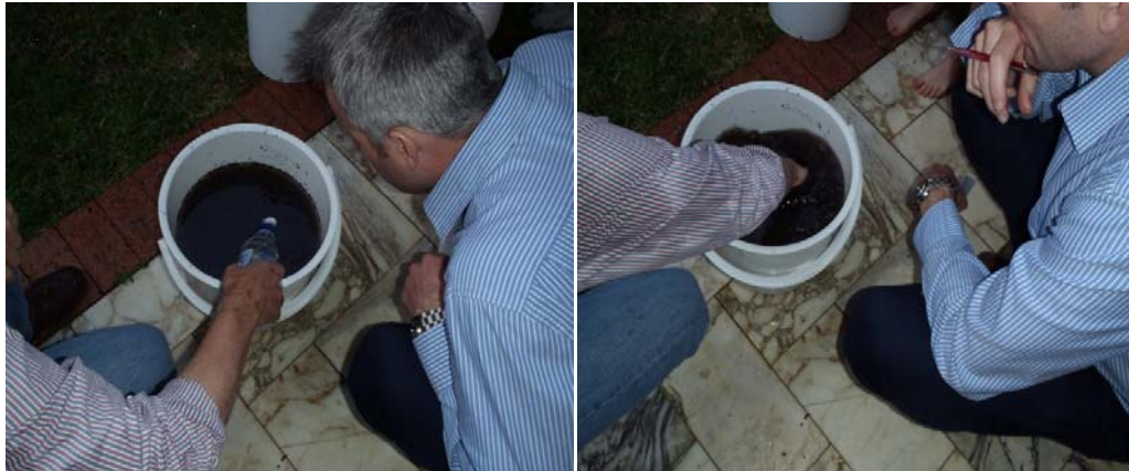
Figure 2 showing pouring in of flocculant and swirling
