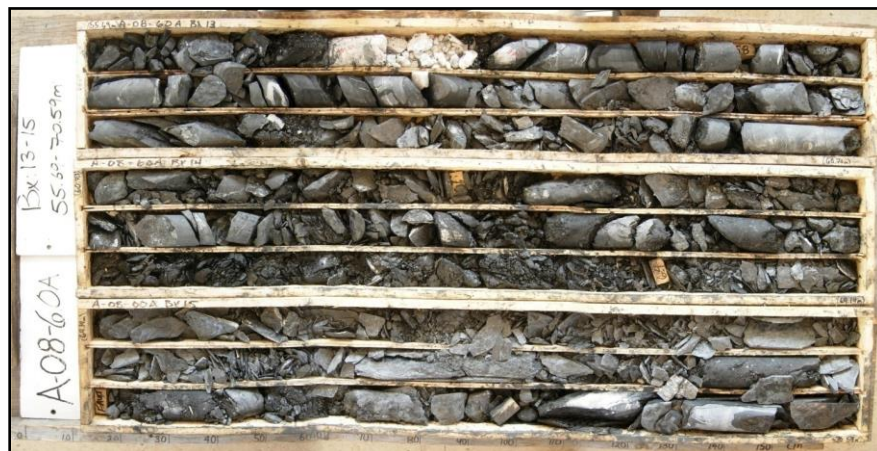
Figure 8-4: Poor ground conditions due to brittle faulting
