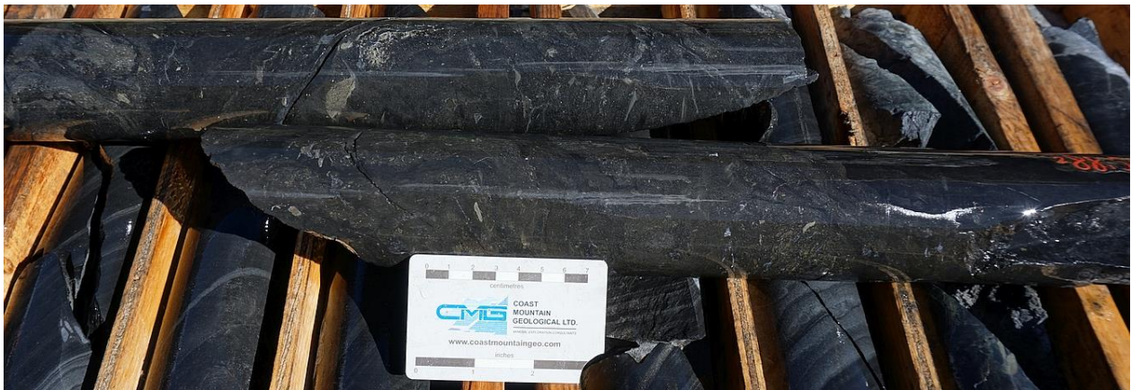
Figure 8-6: An example of previously unrecognised HEBS interval in A-10-72 @ ~288.00m
