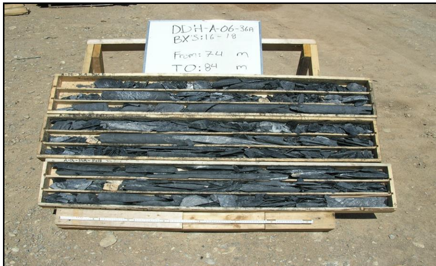
Figure 8-3: Fissile character of the Gunsteel shale
