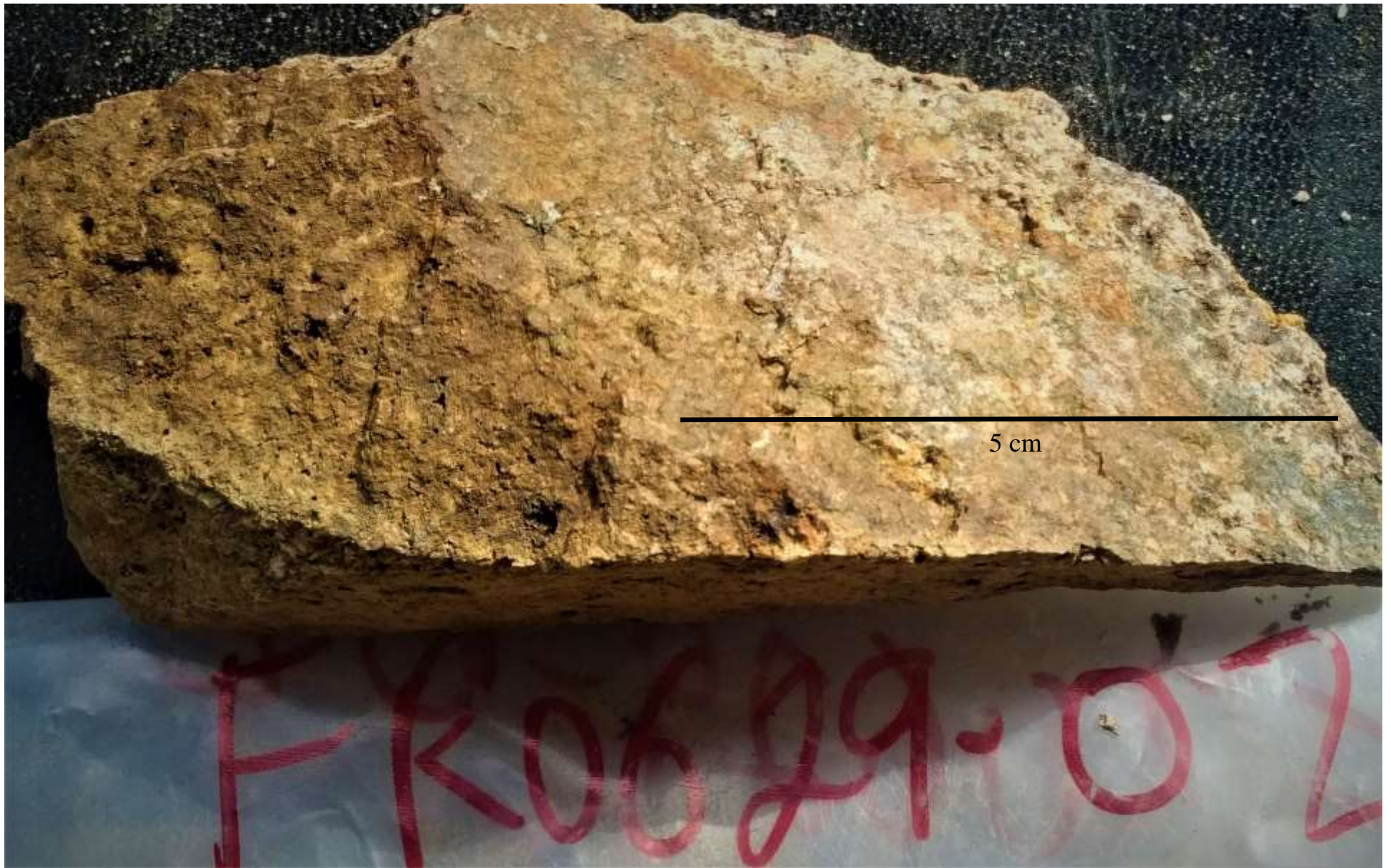
FR0629-02 UTM 682216E 5500325N 1252 EL. Strongly altered and stockwork veined mafic volcanic.
