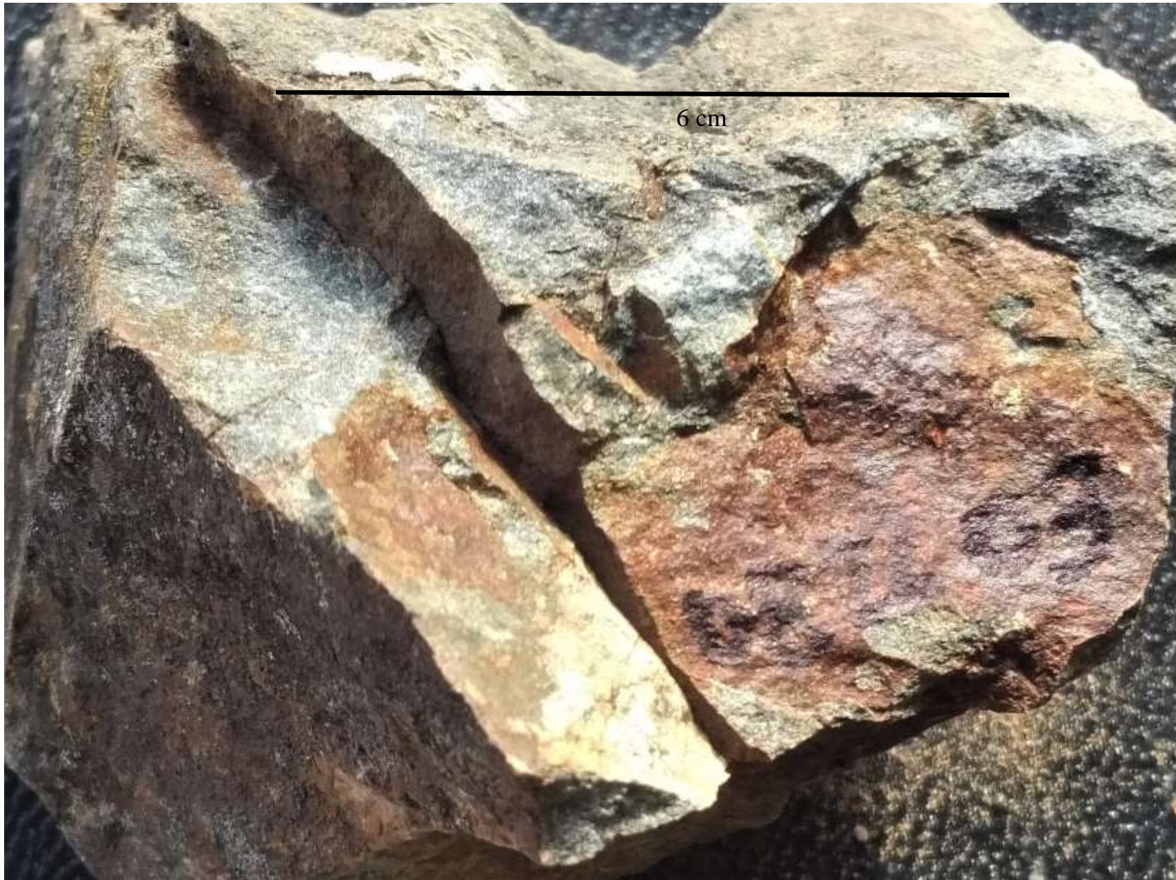
ROC0822-03 UTM 682172E 5500790N 1260 EL. Medium grey-green weathering grey green hornfelsed weakly bleached extremely fine grained volcanic sediment. Moderate bleaching along fractures. Ivory veinlets non-reactive to HCL . Clay? Sediment' hosts moderately strong goethite on weathered fracture coatings. No sulphide noted. Weak magnetic response along some fractures.
