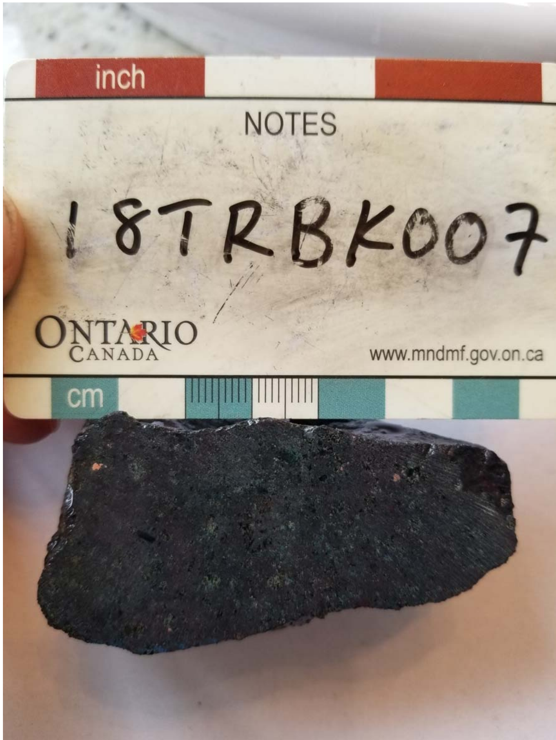
Figure 12: North area native copper bearing, pyroxene-phyric mafic volcanic rock. Millimetre scale blebs of pink coloured native copper are visible in the upper left and upper right of the sample.
