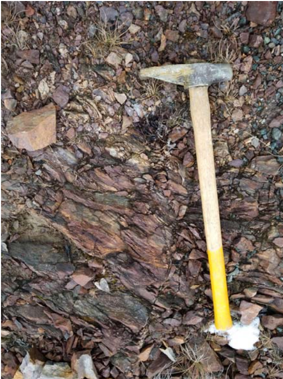
Figure 14: Strongly chlorite-pyrite altered host rocks to the Blacktop showing. Foliation/bedding is oriented 212/25.
