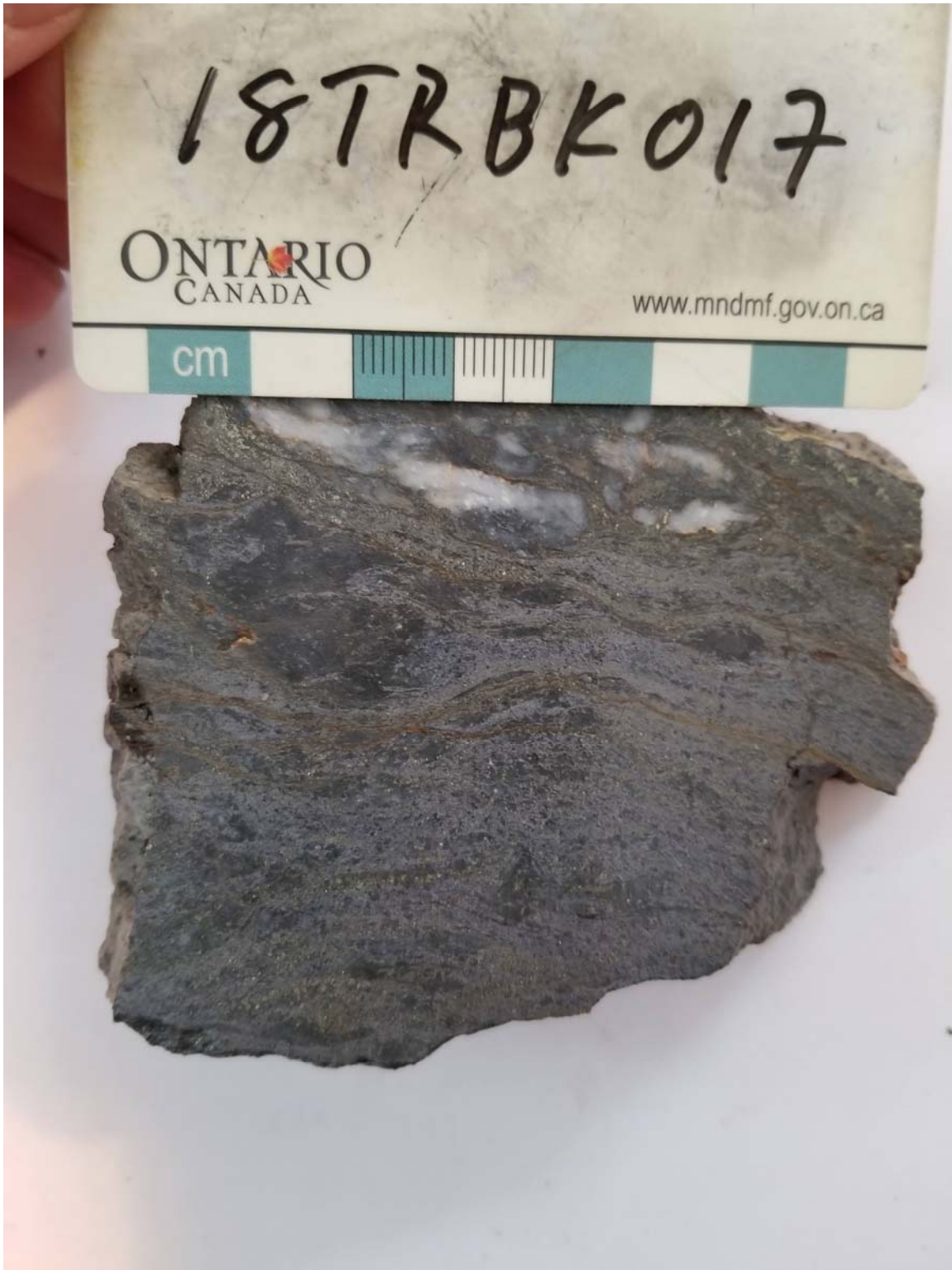
Figure 15: Cut hand sample of VMS mineralization of the Blacktop showing, comprising laminated to thinly bedded layers of fine to very fine grained massive sphalerite, pyrite, and chalcopyrite.
