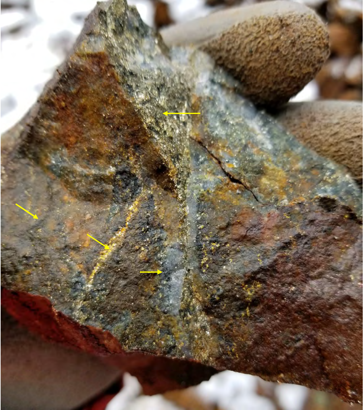
Hand sample from Oxide Creek porphyry showing four stages of veining (station 18JBOP578).
