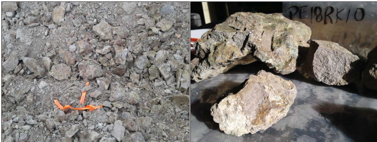
Figure 15 Proof Chip PF18RK10 Sample location (left) and sample (right) crystal tuff-metavolcanic with wavy quartz veins, ankerite selvages, magnetite blotches, pervasive chlorite and green chalcedony pods. Very magnetic.
