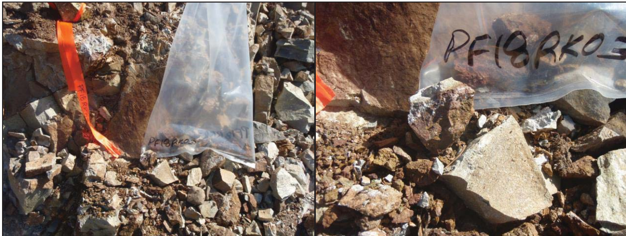
Figure 12 Proof Rock Grab Sample PF18RK03 location (left) and sample (right) – fault gouge with quartz vein with discrete orange crystals in patches of 1.5 cm, Mn-staining and no visible carbonates.
