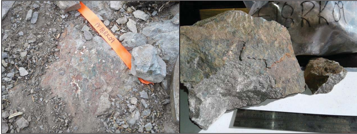
Figure 14 Proof Chip PF18RK09 Sample location (left) and sample (right) crystal tuff-metavolcanic with wavy quartz veins, ankerite selvages, magnetite blotches, pervasive chlorite and green chalcedony pods. Very magnetic.
