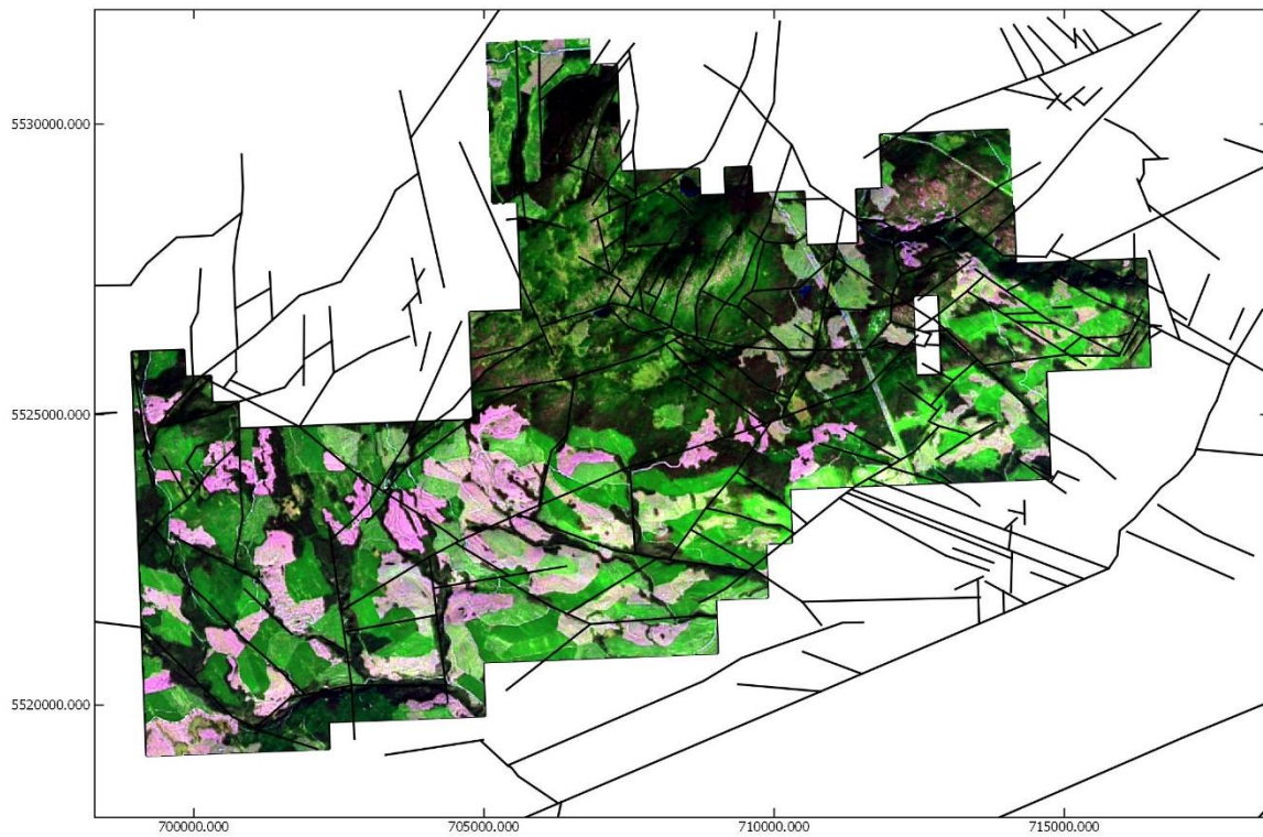
Figure 5. Band combination 7-5-2. This band combination is useful for visualizing different lithologies.
