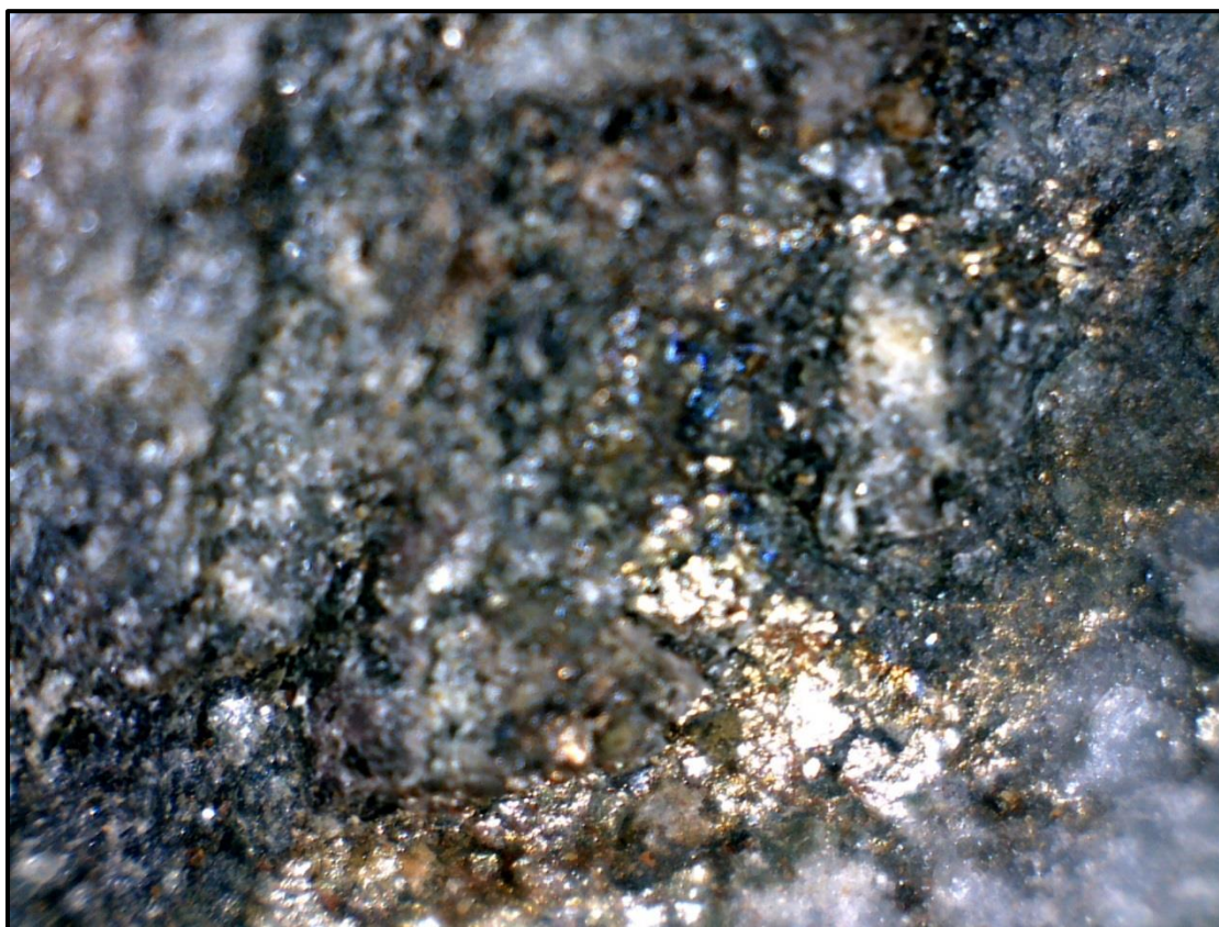
MICROSCOPIC PHOTO 30X CHALCO SPAHLERITE BORNITE SAMPLE T9-R1
