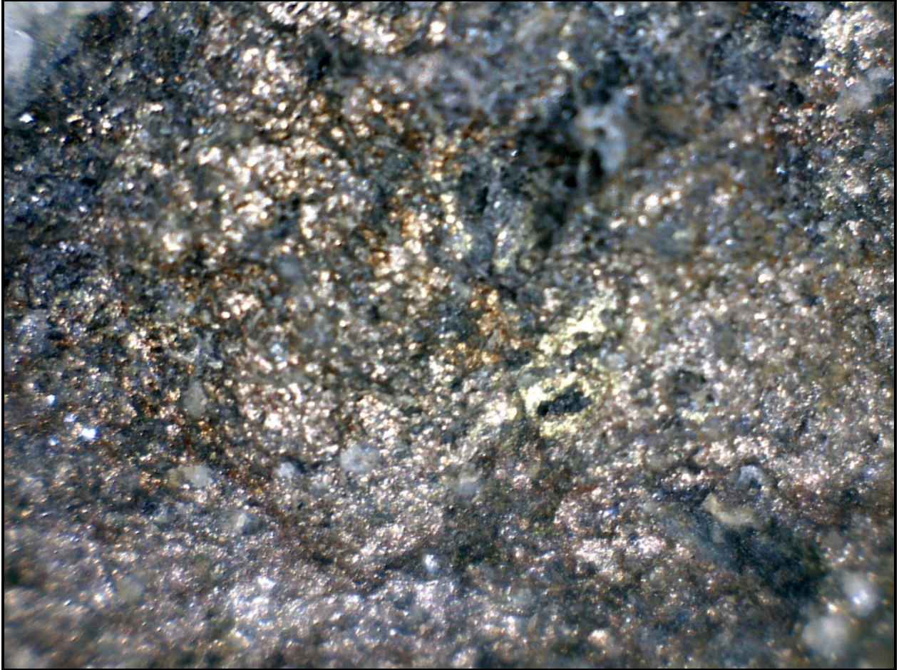
MICROSCOPIC PHOTO 30X CHALCO SPAHLERITE BORNITE SAMPLE T9-R4
