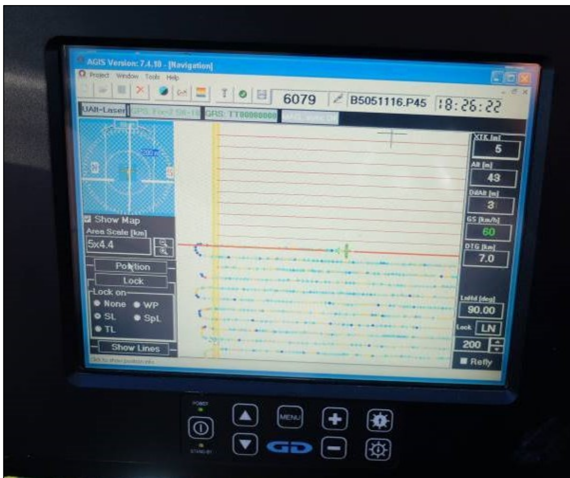
Figure 13: AGIS operator display installed in Airbus AS350 survey helicopter, with screen displaying real time flight line recording and navigation parameters. Additional windows display real time geophysical data to operator.
