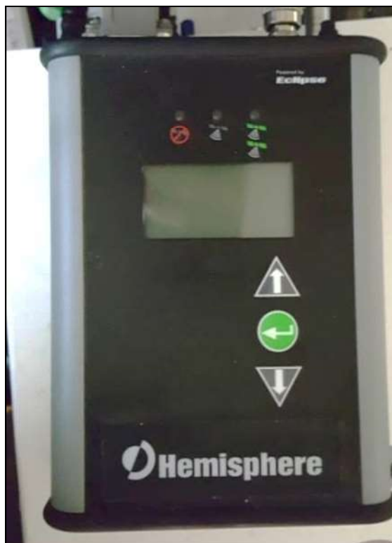
Figure 19: Hemisphere R120 GPS receiver.
