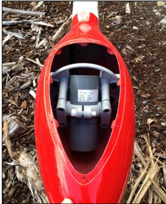
Figure 14: View of cesium vapor magnetometer. Sensor oriented 45° from vertical to couple with local magnetic field at the Windfall Hills survey block.
