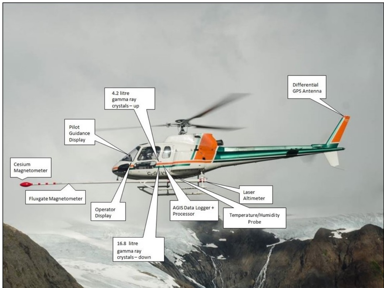
Figure 12: Survey helicopter equipped with geophysical equipment.
