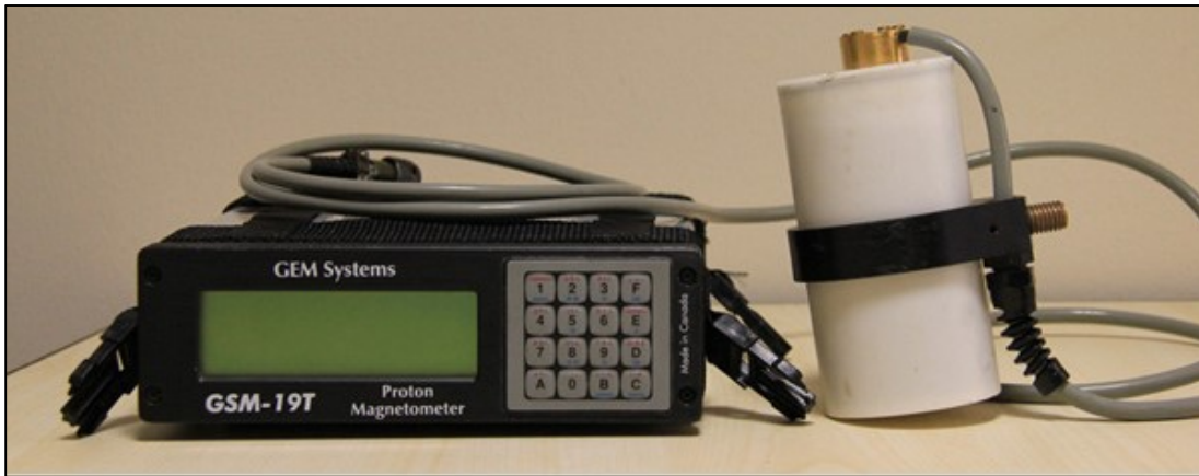
Figure 16: GEM GSM-19T proton precession magnetometer.
