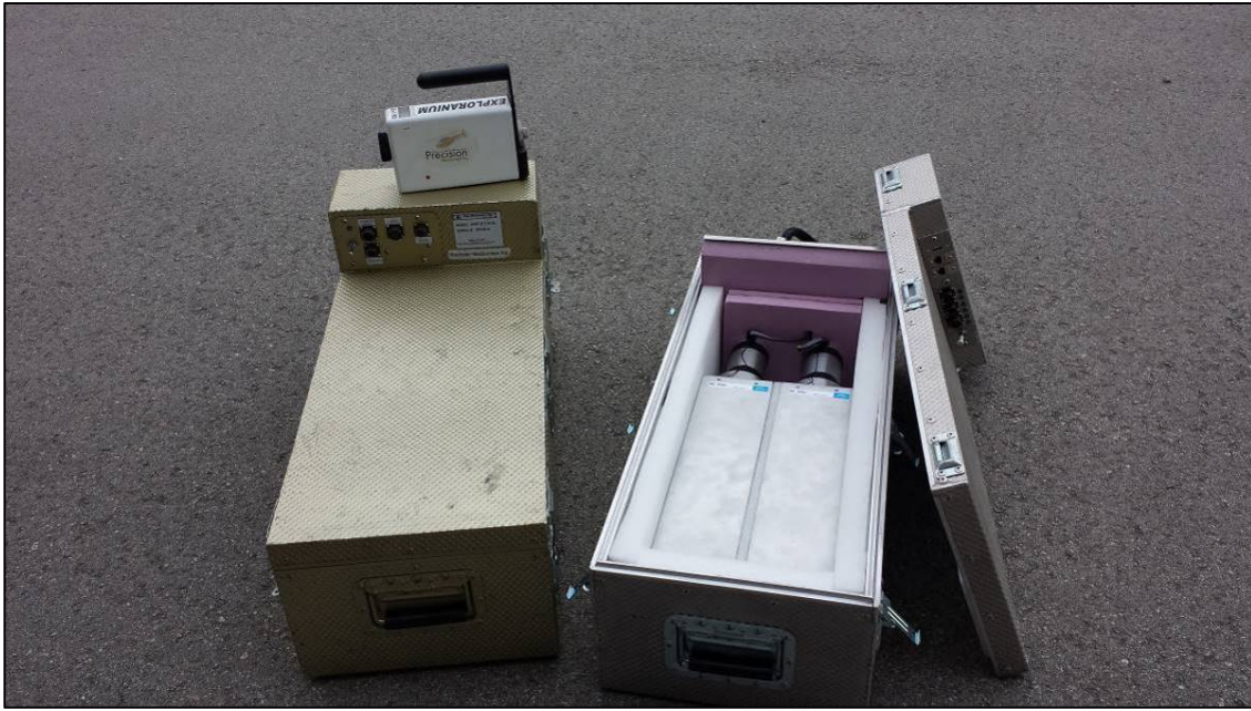
Figure 15: GRS-10 thallium-activated sodium iodide gamma spectrometer crystal packs. The open unit on the right shows two individual 4.2 litre gamma detectors.
