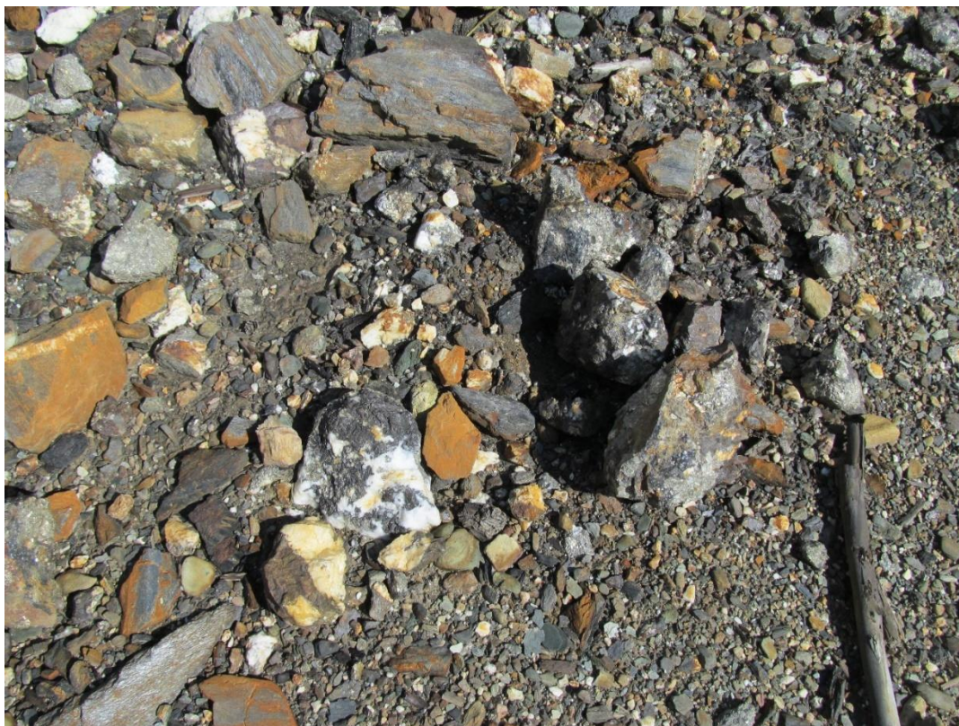
Figure 9: Close-up of representative high grade to ore grade mineralization in stockpiled material
