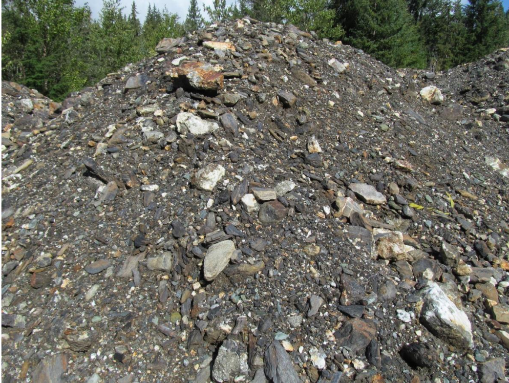
Figure 7: Close-up of representative mixed mineralized and weakly to unmineralized comprising stockpiled material from New Pit Area on Teddy Glacier Showing.
