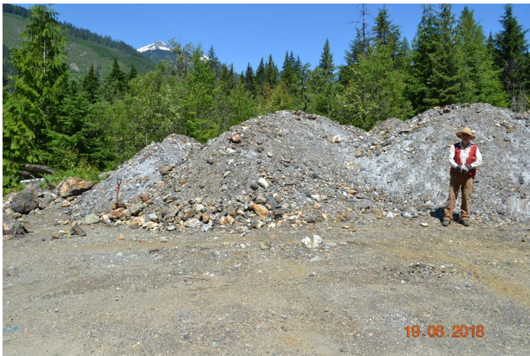
Figure 8: South end of stockpiled material from New Pit area on Teddy Glacier Showing. Stockpile is a mix of medium to high grade ore and weakly to unmineralized material. Geologist for scale.
