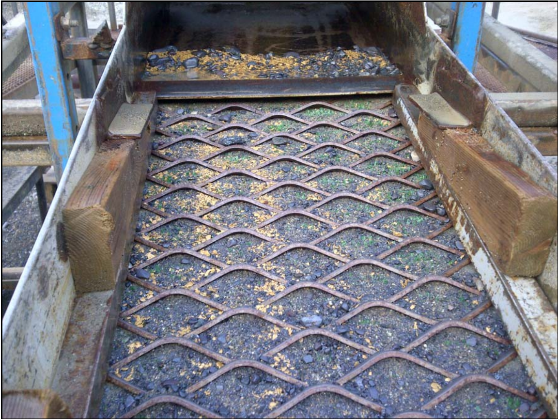
Figure 12 Secondary Plant Sluice No.1, Carpet
