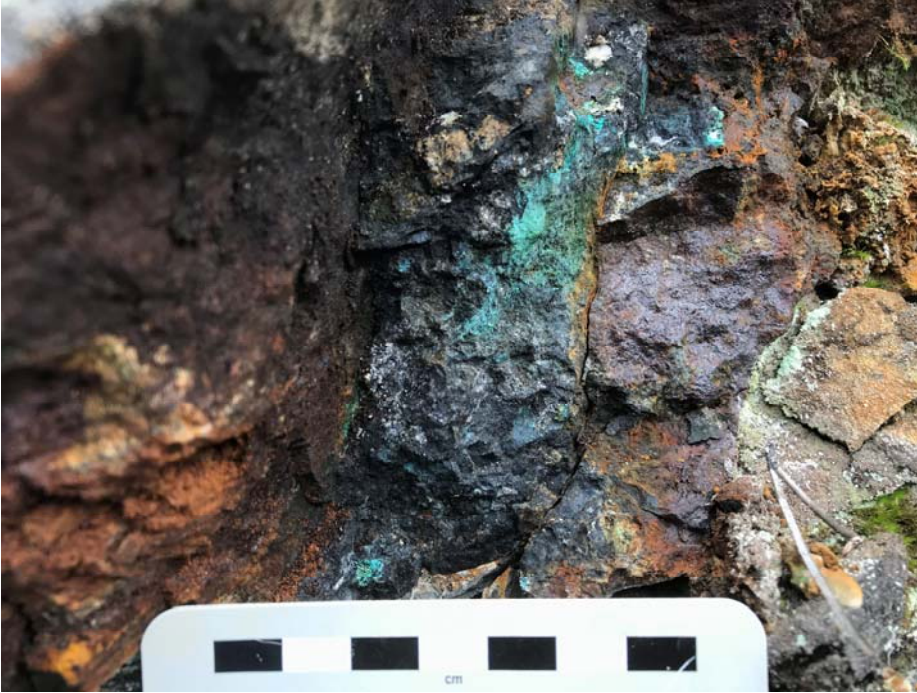
Photo 7: K-feldspar-actinolite?-magnetite-chalcopyrite veins, Vector Zone (sample S849909 - 1.25% Cu).
