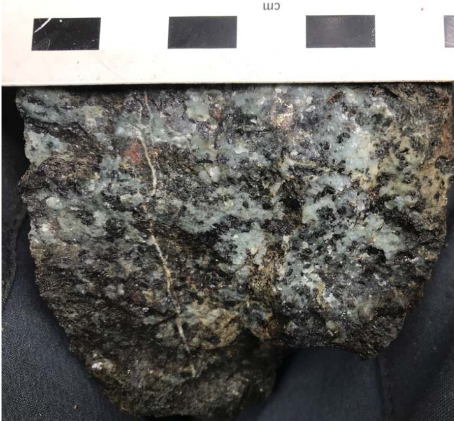
Photo 9: Disseminated chalcopyrite, Mid Zone (sample S849901 - 0.3% Cu).
