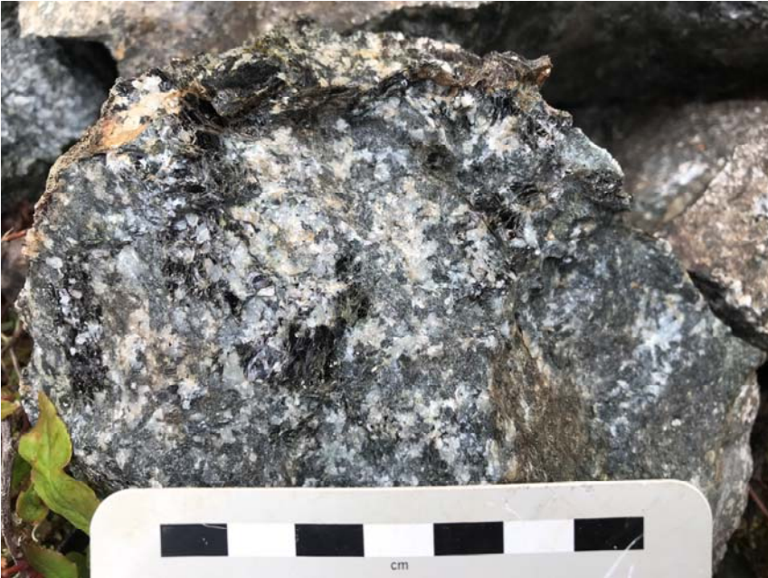
Photo 3: coarse grained granodiorite with coarse biotite (stn EA19SM005).
