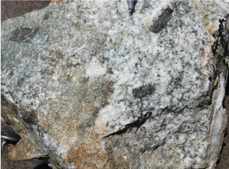
Strongly bimodal amphibole distribution in amphibole-phyric quartz diorite. Note pencil tip for scale.
