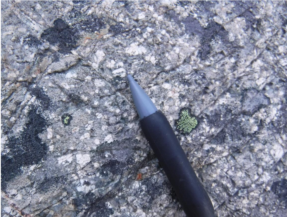
Example of feldspar-phyric porphyry (4naf)
