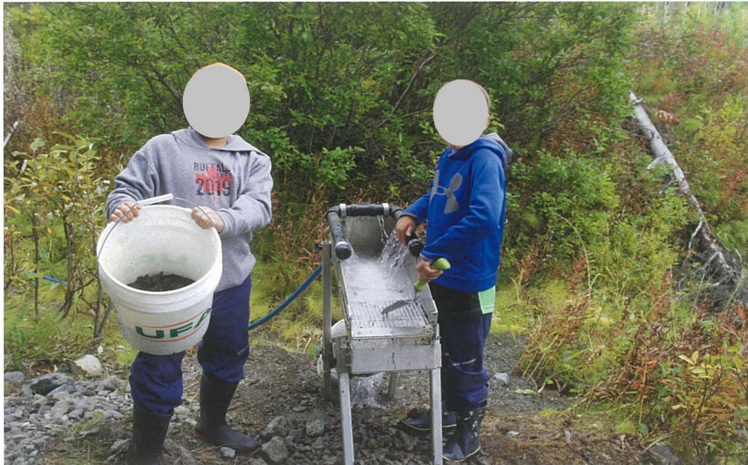
Photo#6. Showing gravel washed residue from high banker ready to be panned. Photo Credit: Quinn Hayden, August 2019.
